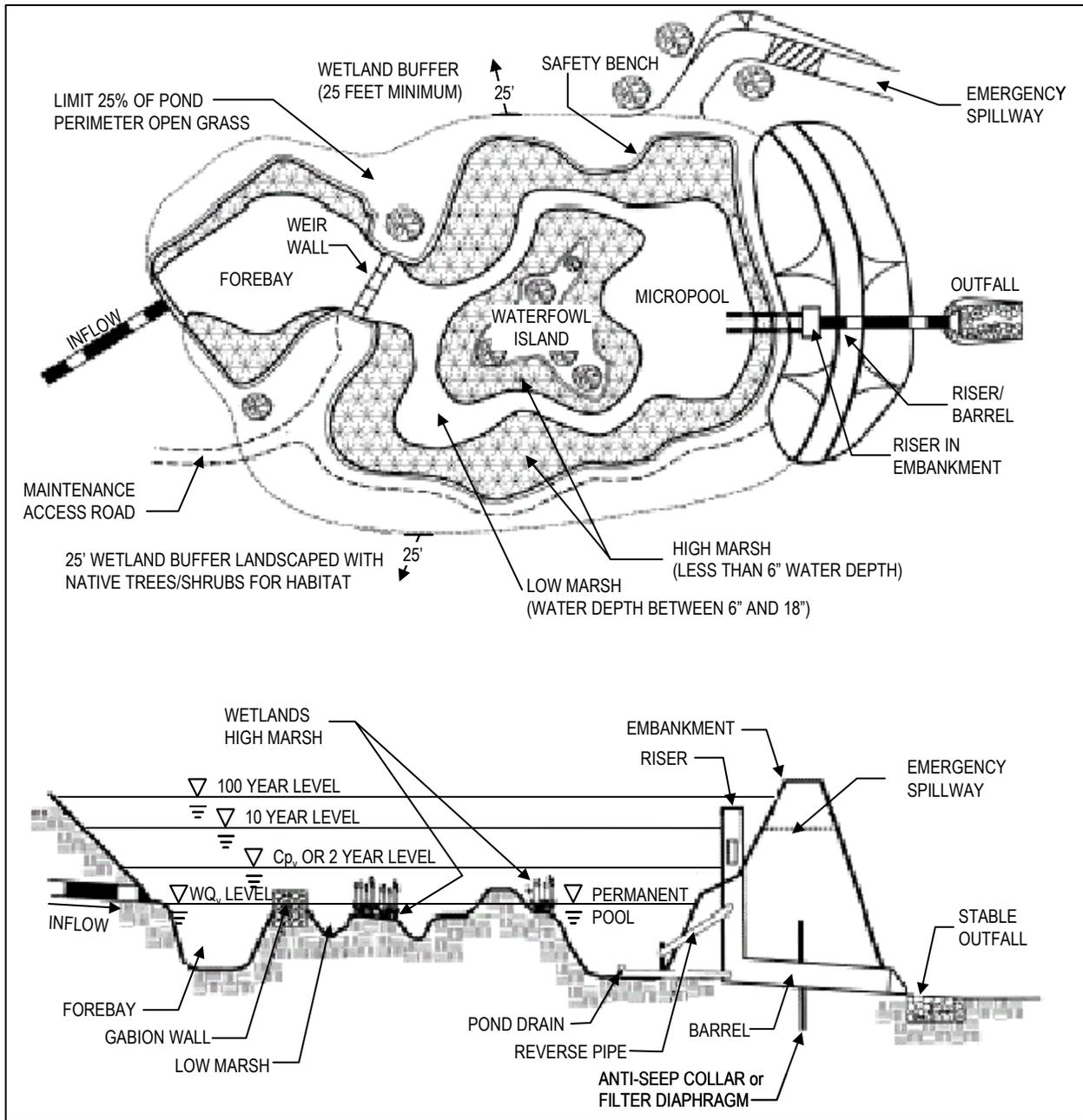
**Figure 5.15: Schematic of a shallow wetland (MDE, 2000).**
