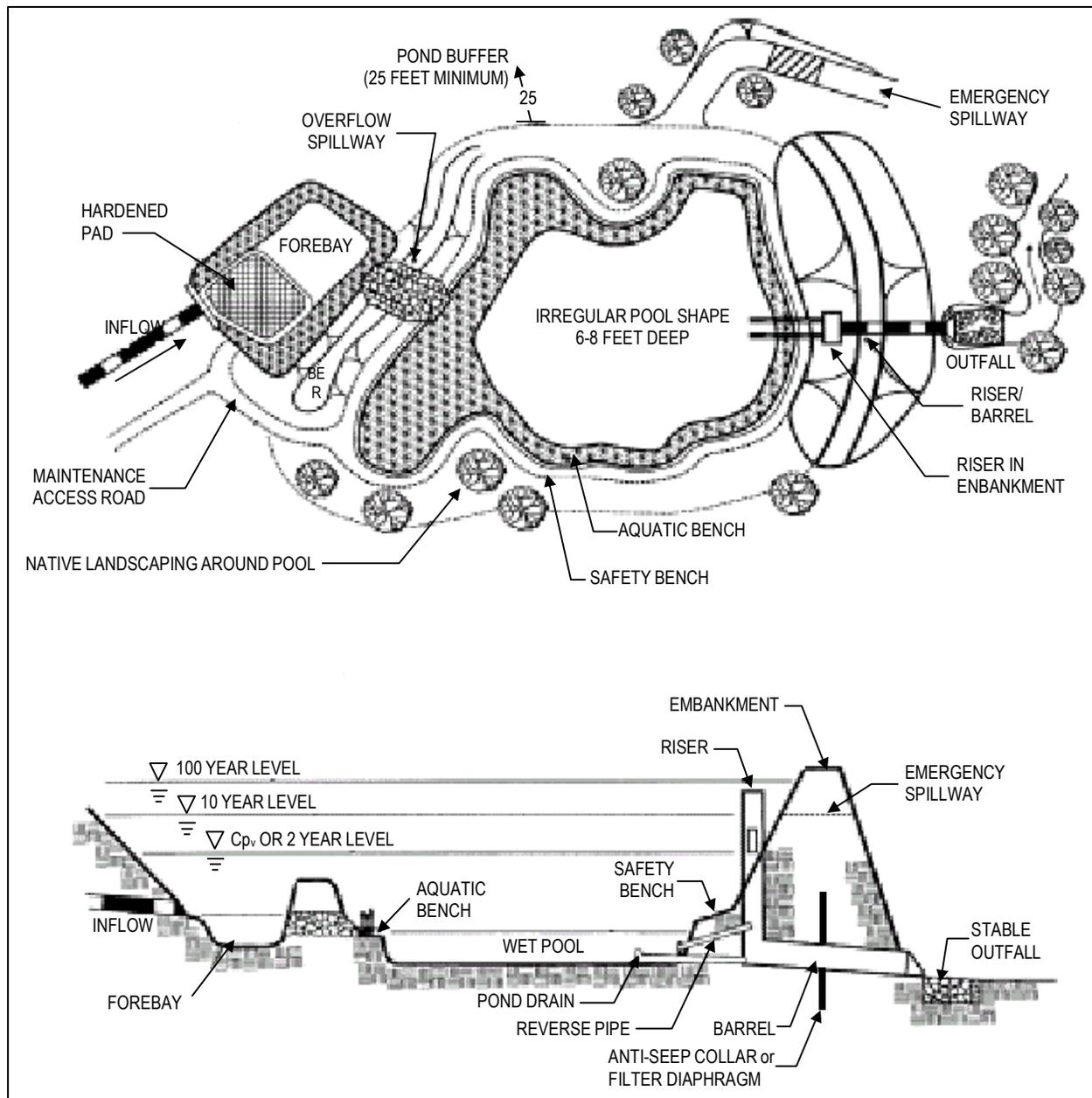
**Figure 5.14: Schematic of a wet pond (MDE, 2000).**
