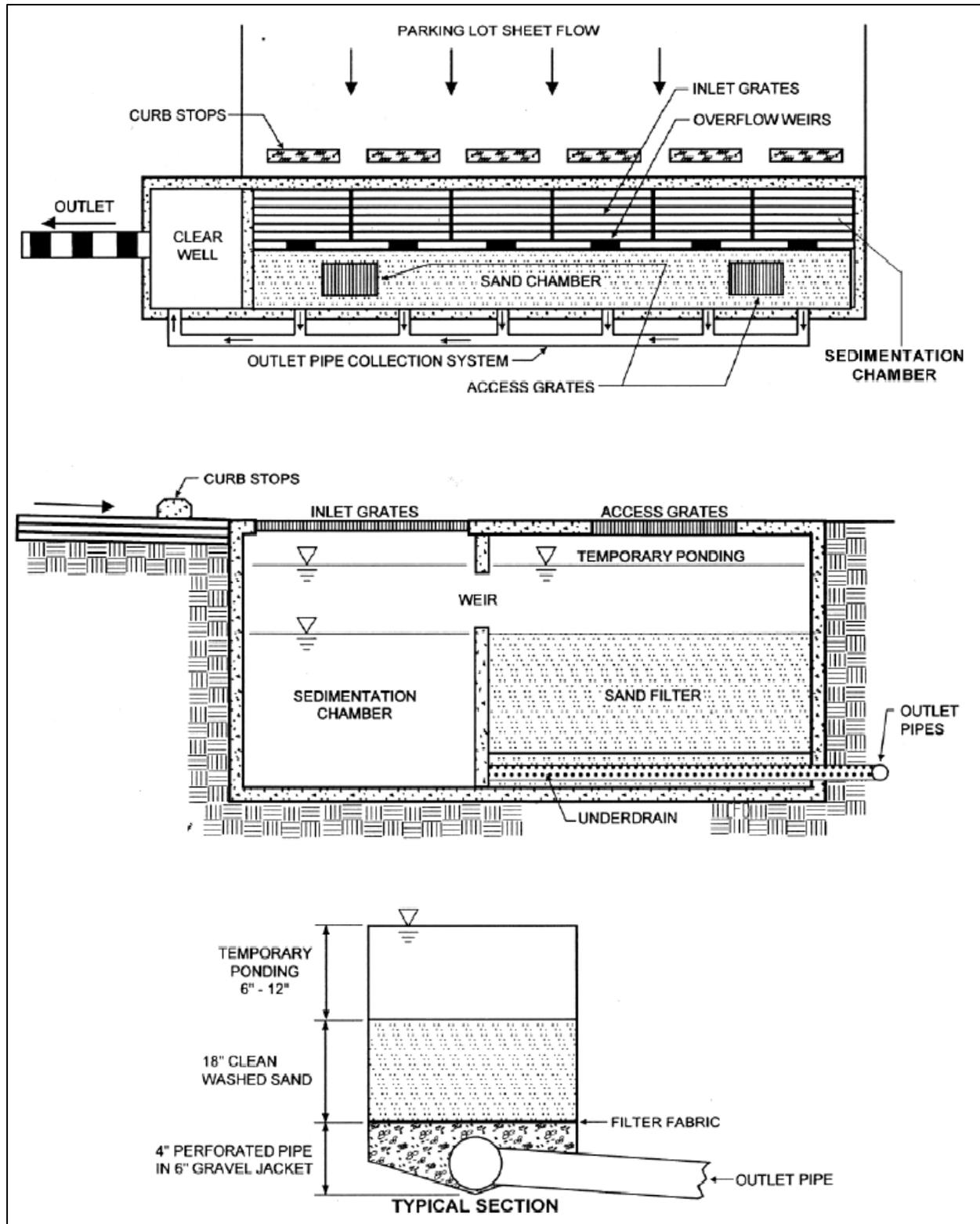
Figure 5.8: Schematic of a perimeter sand filter (MDE, 2000).
