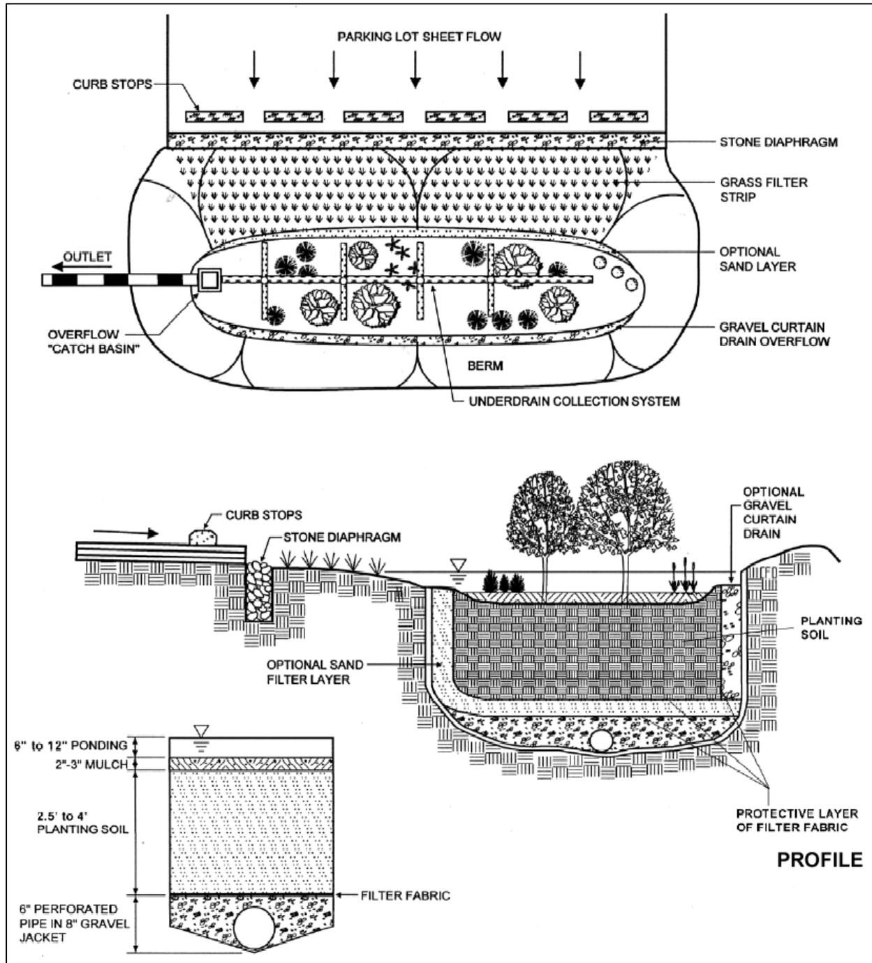
Figure 5.11: Schematic of a bioretention system (MDE, 2000).
