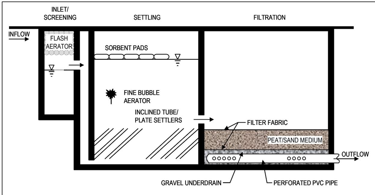
Figure 5.10: Schematic of a multi-chambered treatment train (Pitt, 1996).
