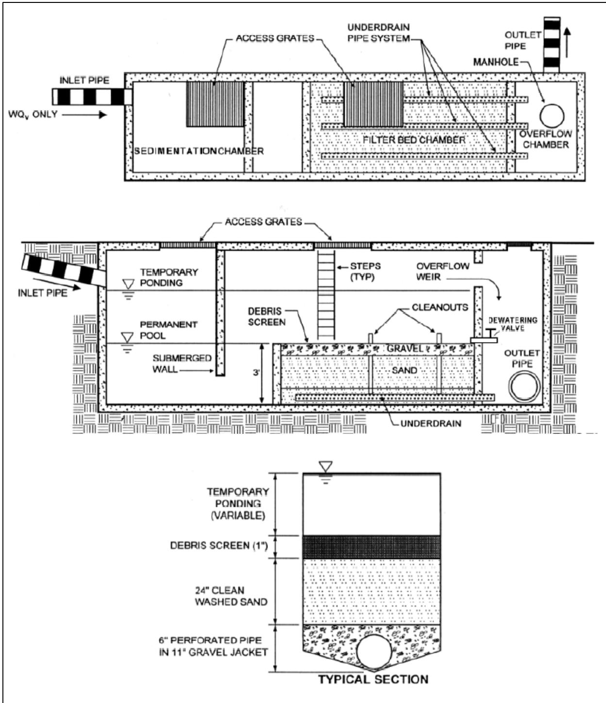
Figure 5.7: Schematic of an underground sand filter (MDE, 2000).
