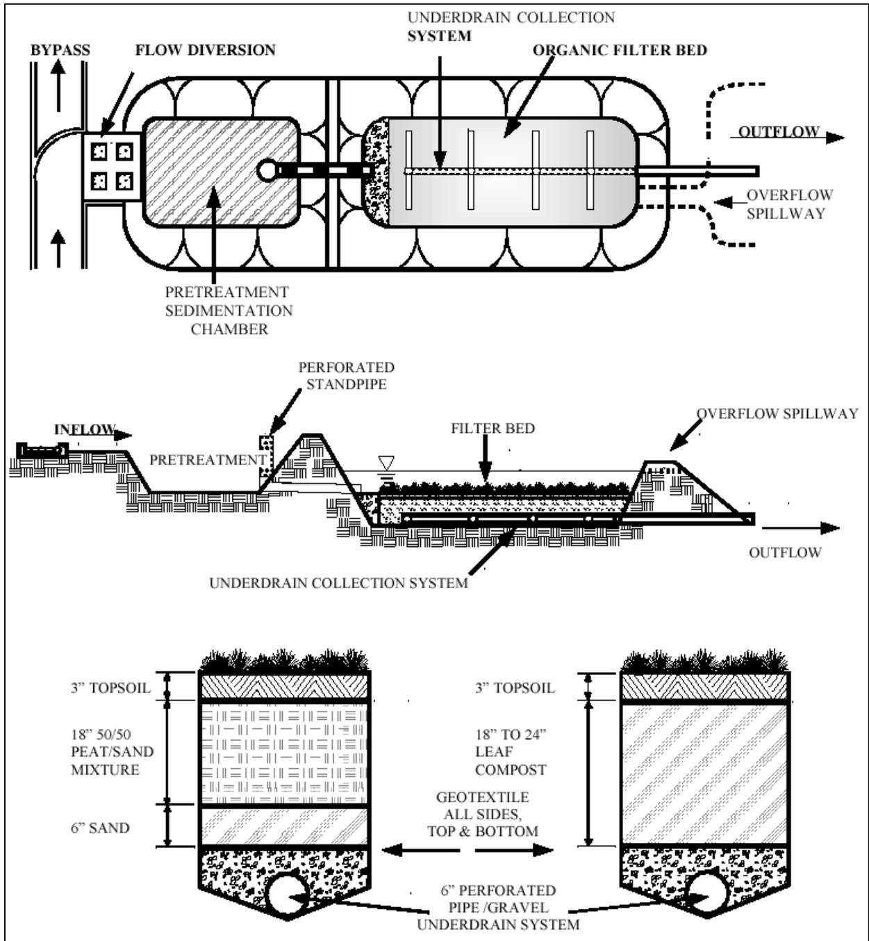
Figure 5.9: Schematic of an organic media filter (MDE, 2000).
