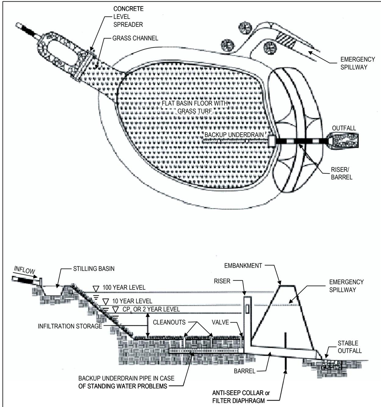
Figure 5.1: Schematic of an infiltration basin (MDE, 2000).
