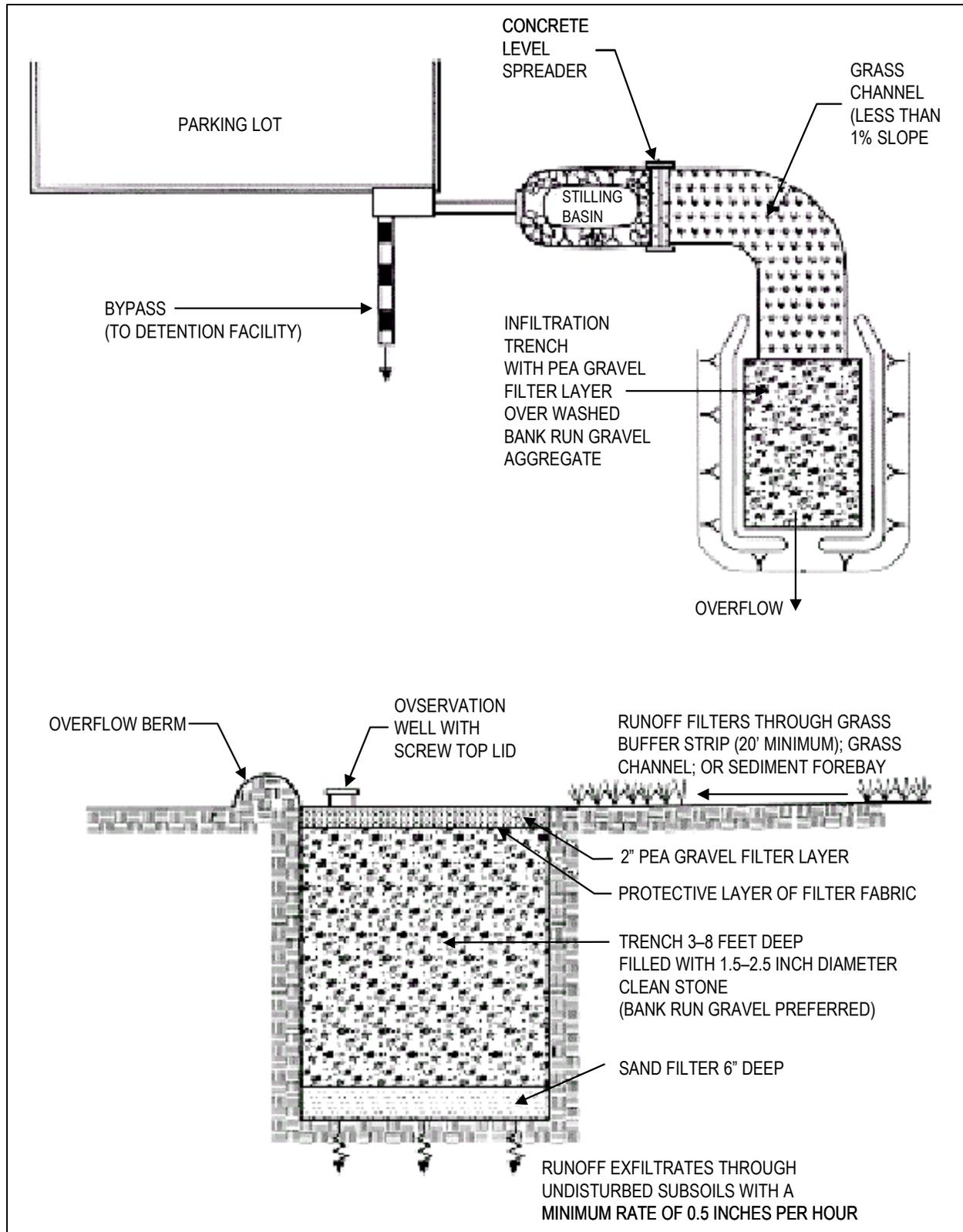
Figure 5.2: Schematic of an infiltration trench (MDE, 2000).
