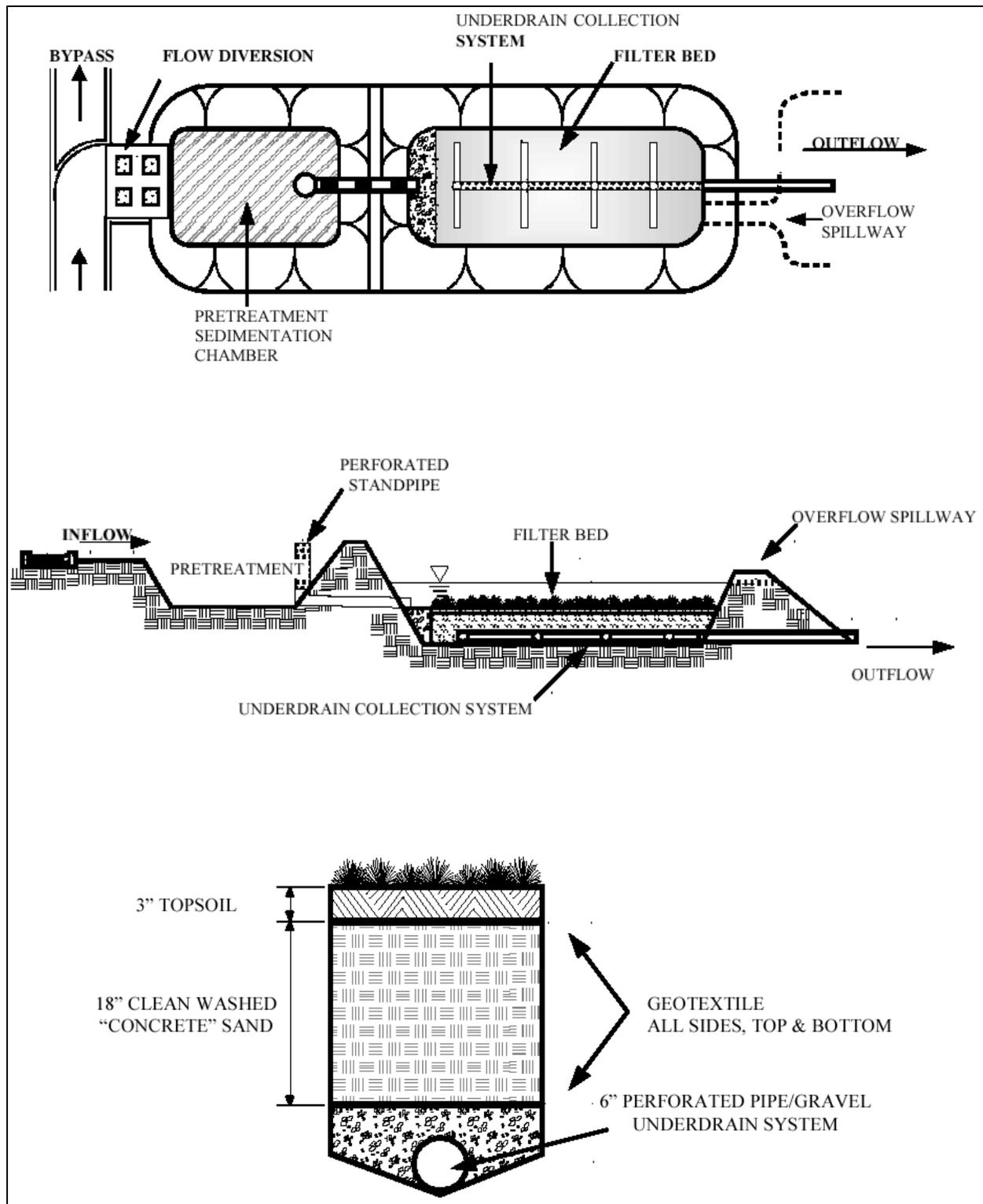
Figure 5.6: Schematic of a surface sand filter (MDE, 2000).
