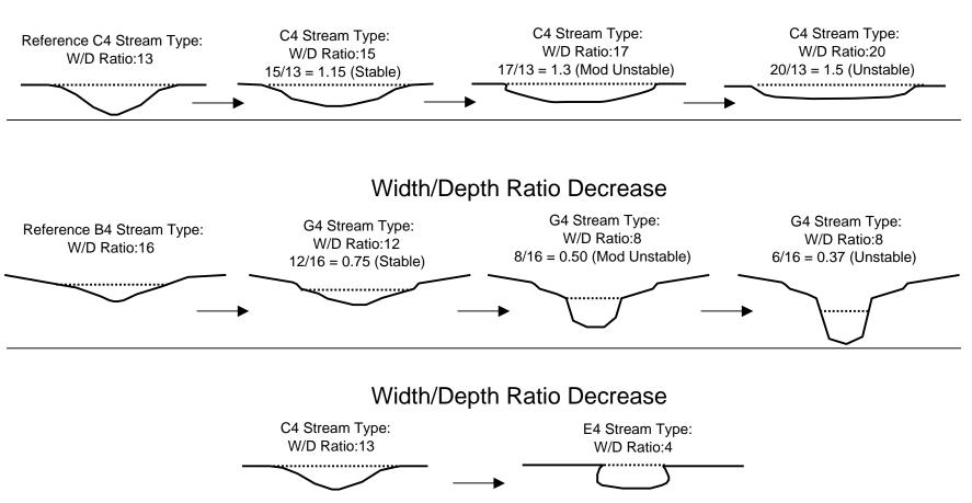
A width/depth ratio decrease is a trend toward stability and/or an evolution to a stable stream type when the bank height ratio is equal to one.
