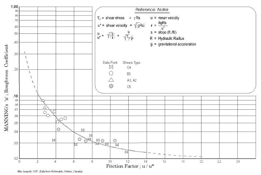
Figure 104. Conversion of a resistance (friction) factor to Manning's "n" roughness coefficient (Leopold, et al, 2000)
