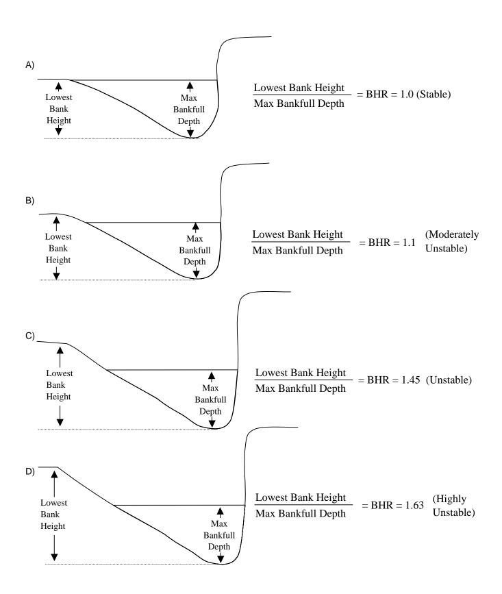
Figure 110. Examples of Bank Height Ratio (BHR) Categories for Stability Evaluation.
