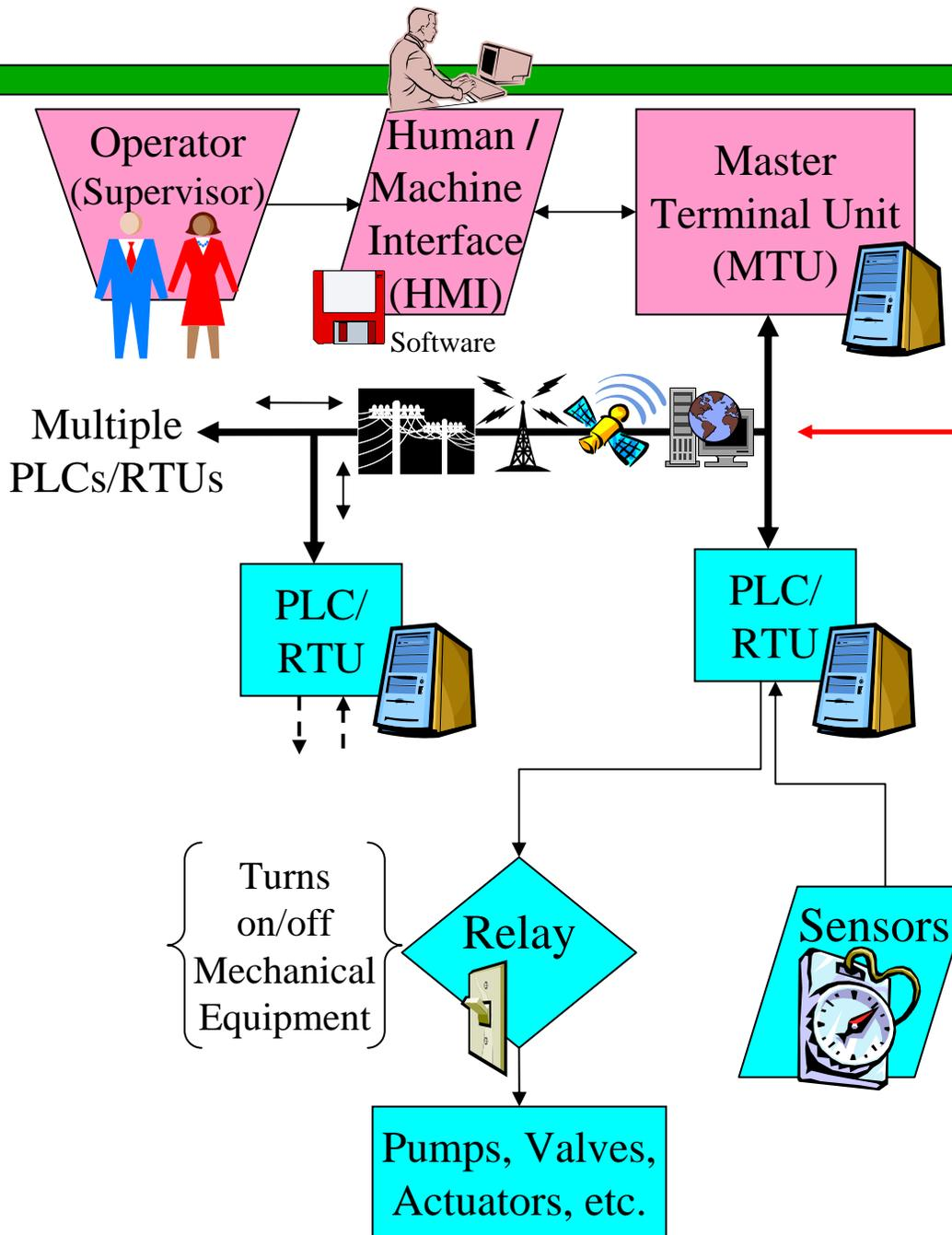
In the early stages utilities ran wires, also known as hardwire or land lines, from the central computer (MTU) to the remote computers (RTUs).
