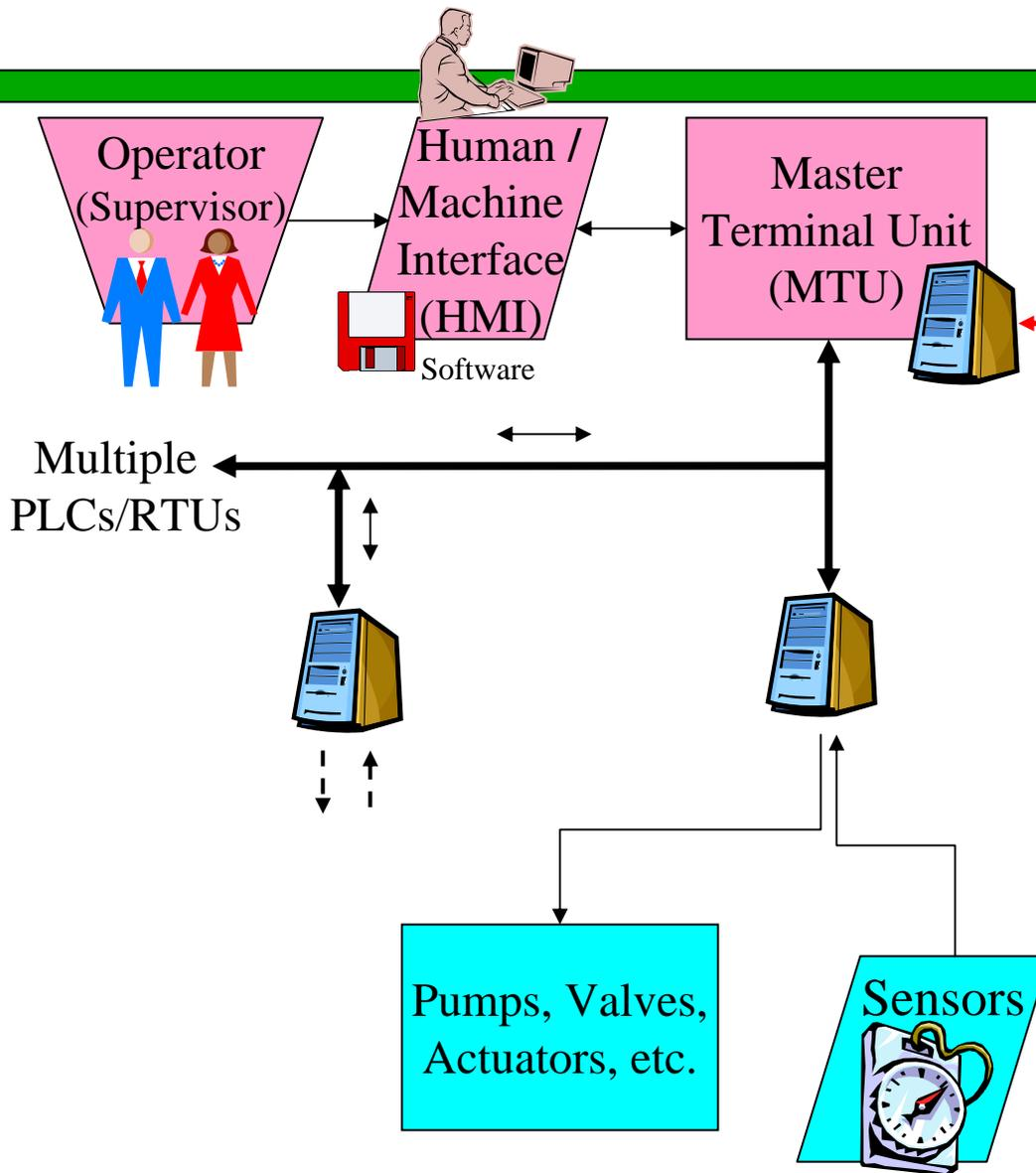
The central computer is called the **Master Terminal Unit, or MTU**. The Operator interfaces with the MTU using a software called Human Machine Interface, or HMI.
