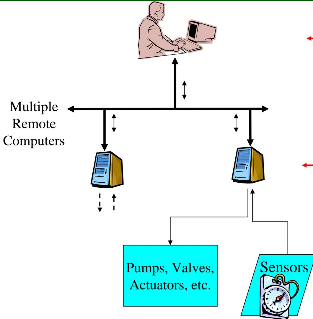
**SCADA** allows an Operator using a central computer to supervise (control and monitor) multiple networked computers at remote locations.
