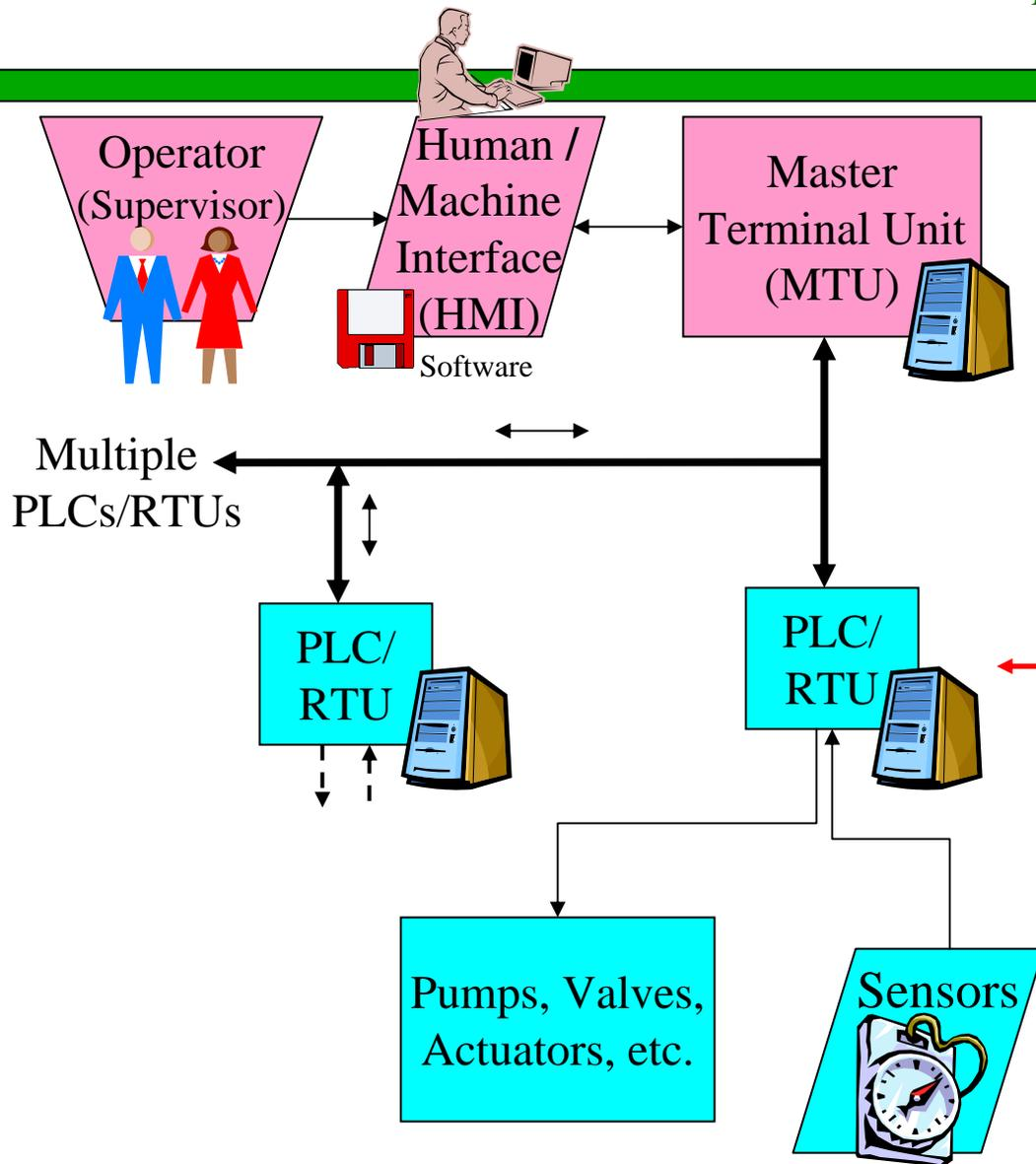
The remote computer is called **Program Logic Controller (PLC)** or **Remote Terminal Unit (RTU)\***
