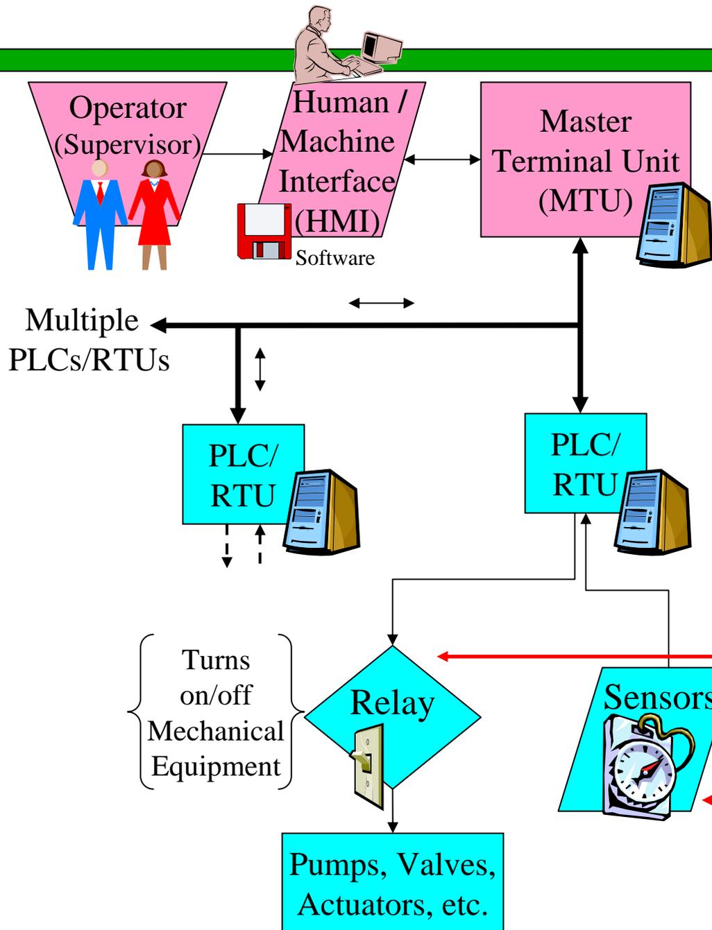
The **RTU** activates a **relay** (or switch) that turns mechanical equipment “on” and “off.” The RTU also collects data from **sensors**.
