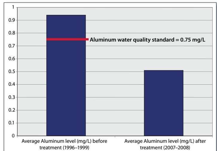
Figure 3. Aluminum reductions in Gumboot Run in milligrams per liter (mg/L).
