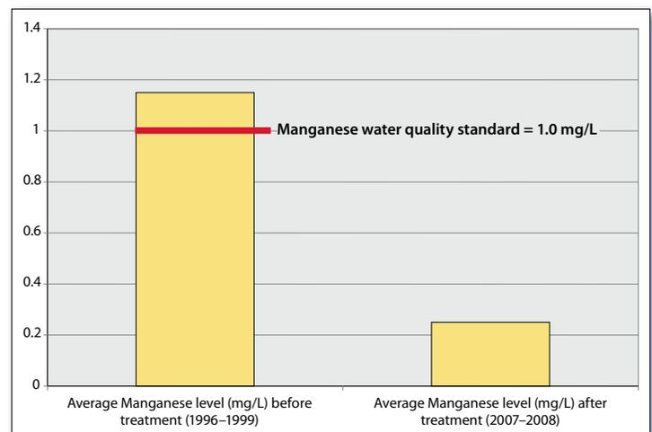
Figure 4. Manganese reductions in Gumboot Run in mg/L.
