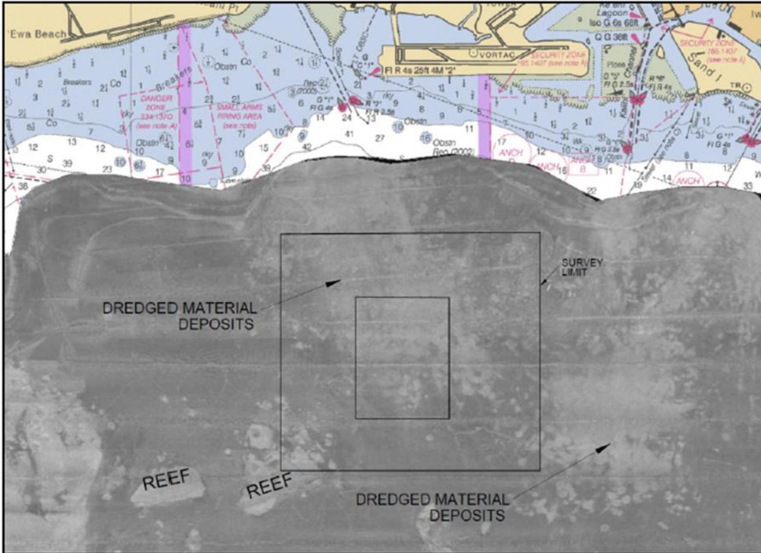
**Figure 27. Transect lines for the sub-bottom profiling survey of the South Oahu site.** Results for Diagonal line 1 through the center of the disposal site (arrows) are given in Figure 29. (Sea Engineering, 2014)
