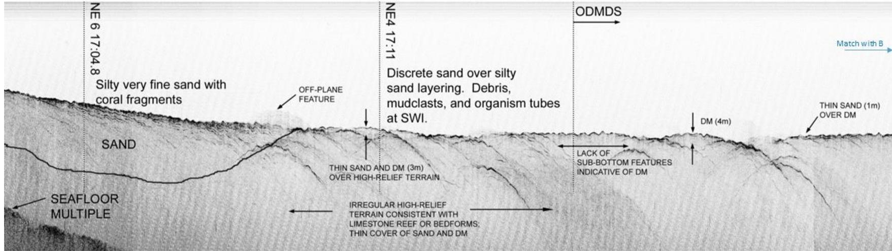
**Figure 29B. Sub-bottom profile – SW portion of Diagonal Line 1.** (Sea Engineering, 2014)
