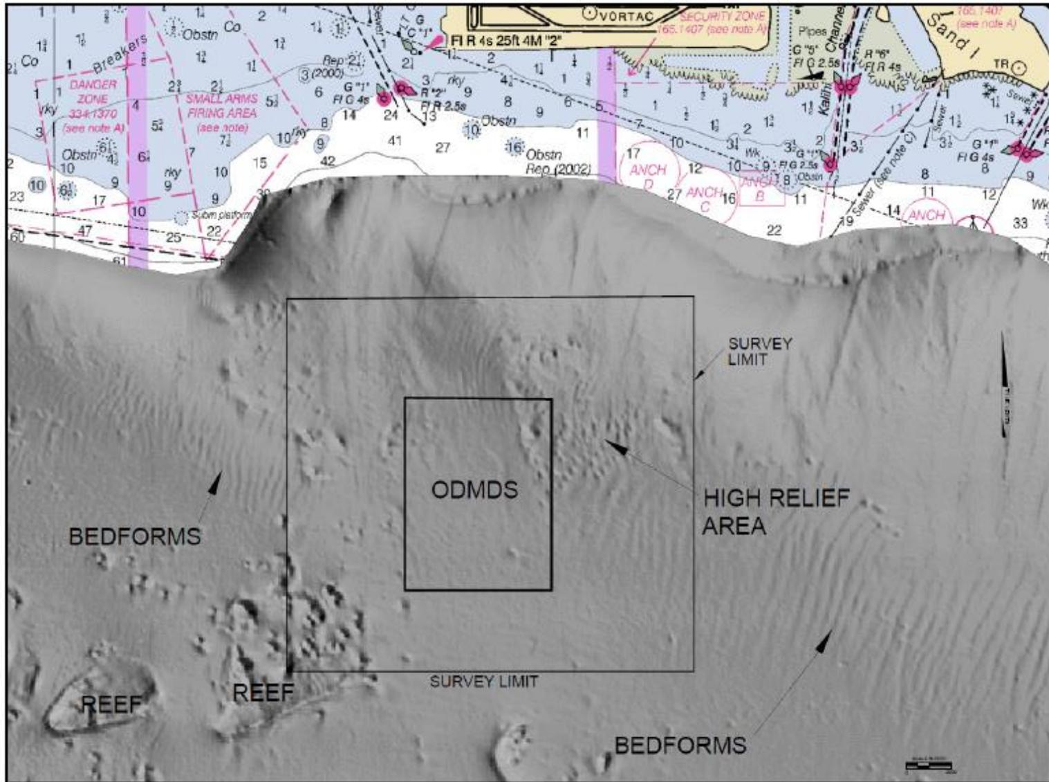
**Figure 26. USGS sidescan sonar (backscatter) image showing historic dredged material deposits around the sub-bottom survey area and the South Oahu disposal site (sidescan imagery from USGS, 2000). (Sea Engineering, 2014)**
