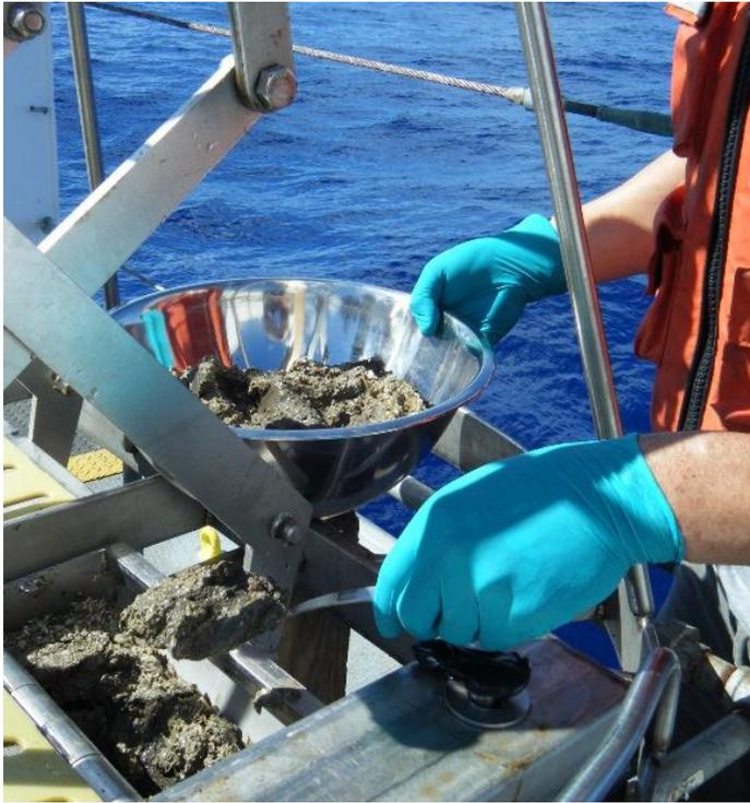
**Figure 11. Processing a sediment sub-sample for chemical analysis.**
