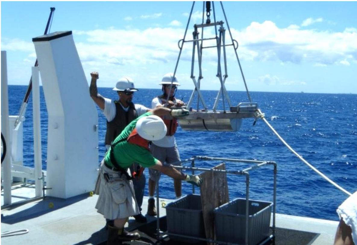
**Figure 10. Subsampling from the Van Veen grab for sediment chemistry.**
