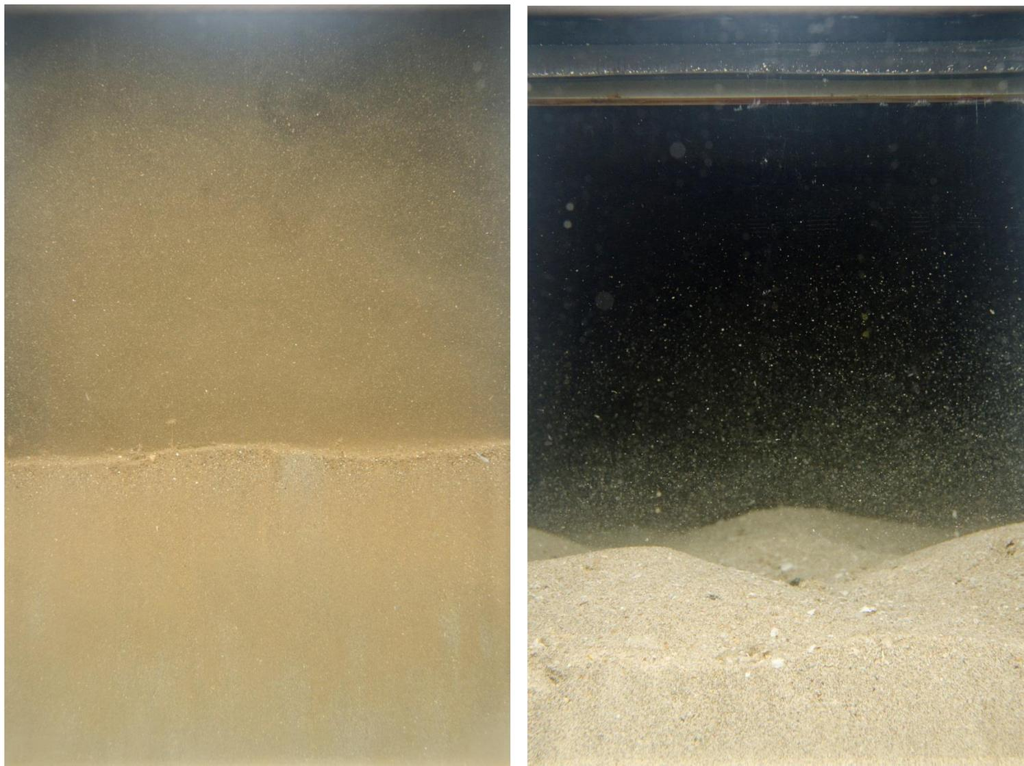
**Figure 16. Plan view images of the dredged material deposit compared to the native seafloor at South Oahu.** Station C1 on dredged material (top) shows the visual difference in both sediment color and surface texture/features of dredged material compared to the ambient bottom at Station NW6 (bottom). Scale: width of each PV image is approximately 4 m. (Germano & Assoc., 2013)
