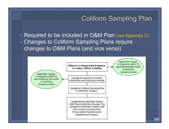
Coliform sampling plans must be included in aircraft water system O&M plans. Any changes made to coliform sampling plans require changes to O&M plans, and vice versa.
