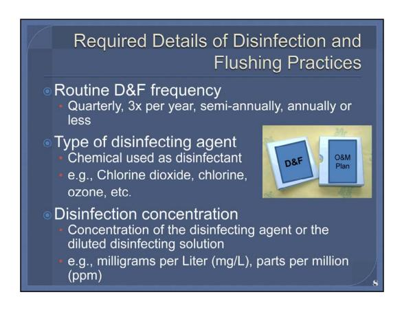
Specifically, the ADWR requires that the O&M plan identify the following details of disinfection and flushing practices [40 CFR 141.804(b)(2)]. These are to be based on the water system manufacturer's recommendations, when available. The disinfection and flushing frequency may be quarterly, three times per year, semi-annually, or annually or less than annually. Of course, the less frequently that D&F is performed, the more frequently routine coliform samples must be sampled.
