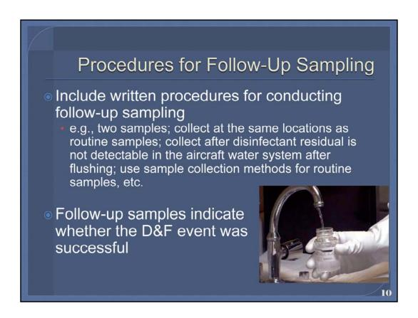
The O&M plan must include written procedures for conducting follow-up coliform sampling after a corrective disinfection and flushing event takes place. Follow-up samples indicate whether the disinfection and flushing event was successful.
