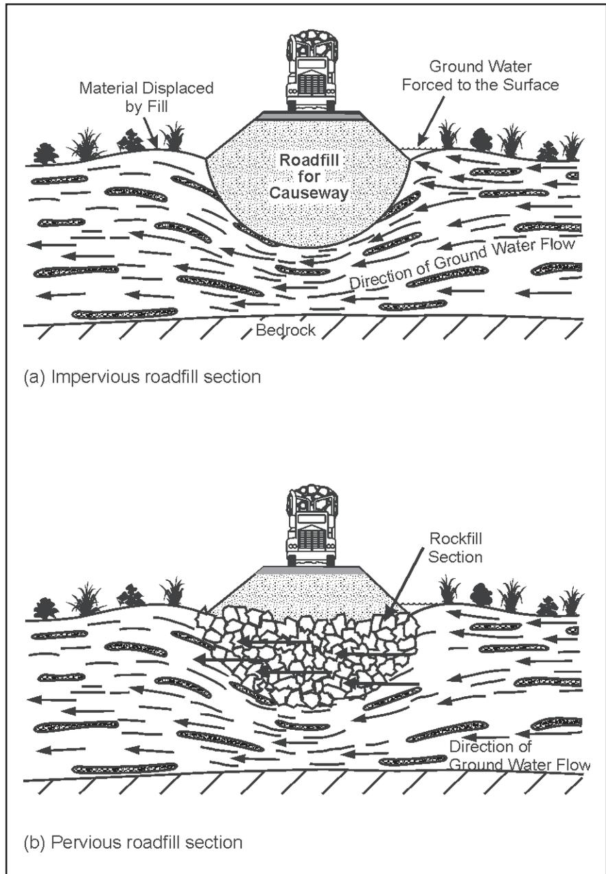
**Figure 3-46. Comparison of impervious (a) and pervious (b) roadfill sections. Impervious roadfill consolidates natural material and restricts groundwater flow. Pervious roadfill allows movement of groundwater through it and minimizes flow changes (adapted from Thronson, 1979).**
