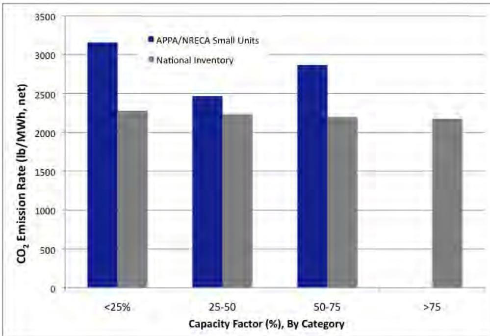
Figure 3-5. CO<sub>2</sub> Emission Rates for Small EGUs vs. National Inventory, By Quartiles of Capacity Factor
