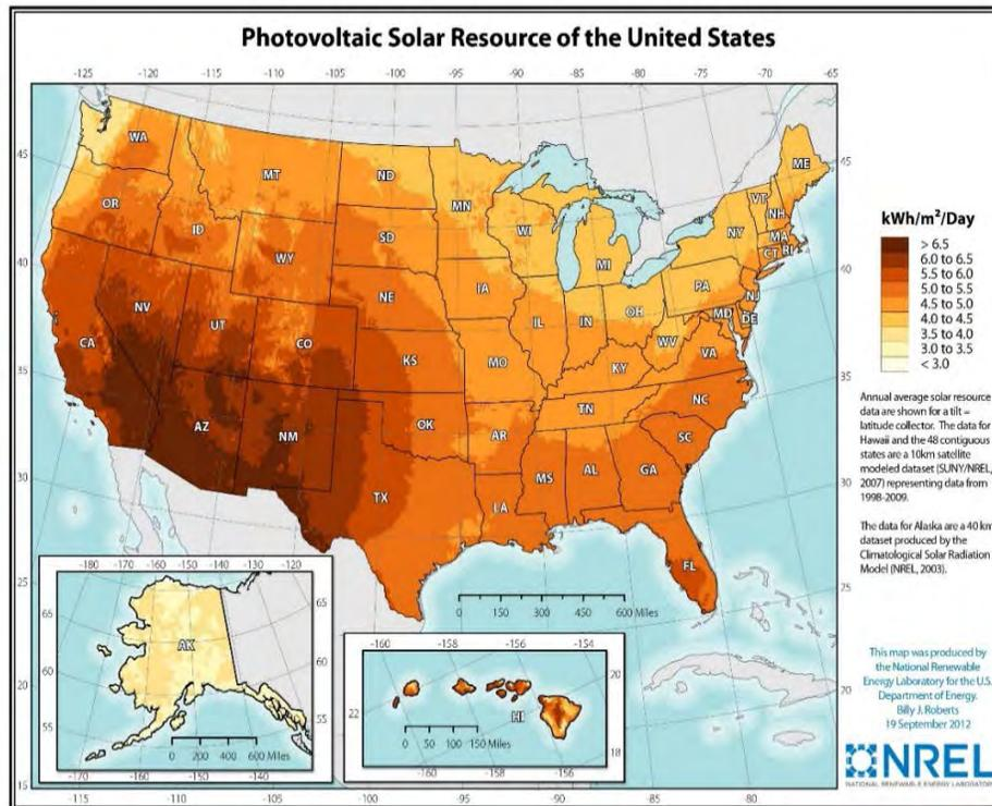
Figure 3 U.S. Solar Photovoltaic Resource Map, Using Data from 1998 to 2009 Regions with darker color indicate higher potential or photovoltaic solar power generation
