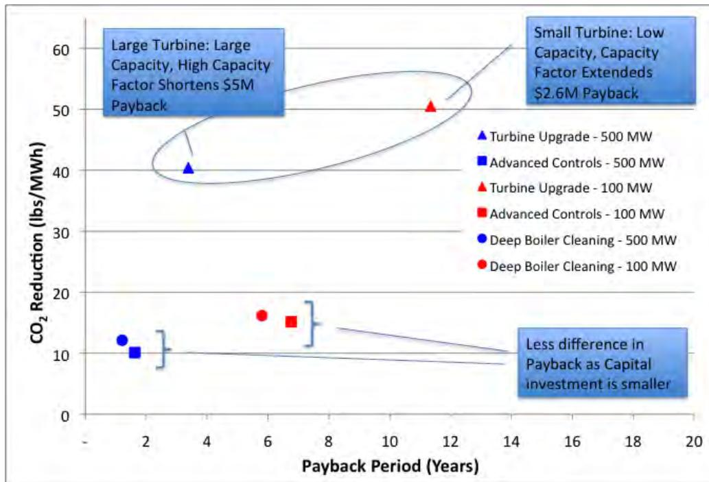
Figure 5-2. CO<sub>2</sub> Reduction vs. Calculated Payback Period
