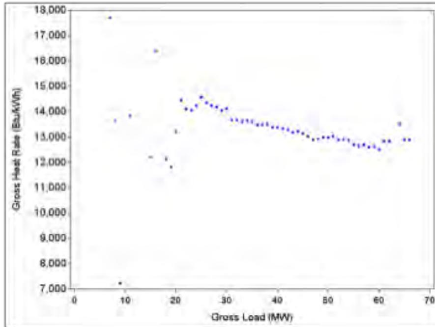
Figure A-1. Gross Plant Heat Rate vs. Load: CR Lowman Unit 1
