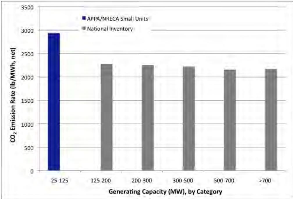
Figure 3-3. CO<sub>2</sub> Emission Rates by Categories of Generating Capacity (MW): Small APPA/NRECA EGUs, 2007 - 2013
