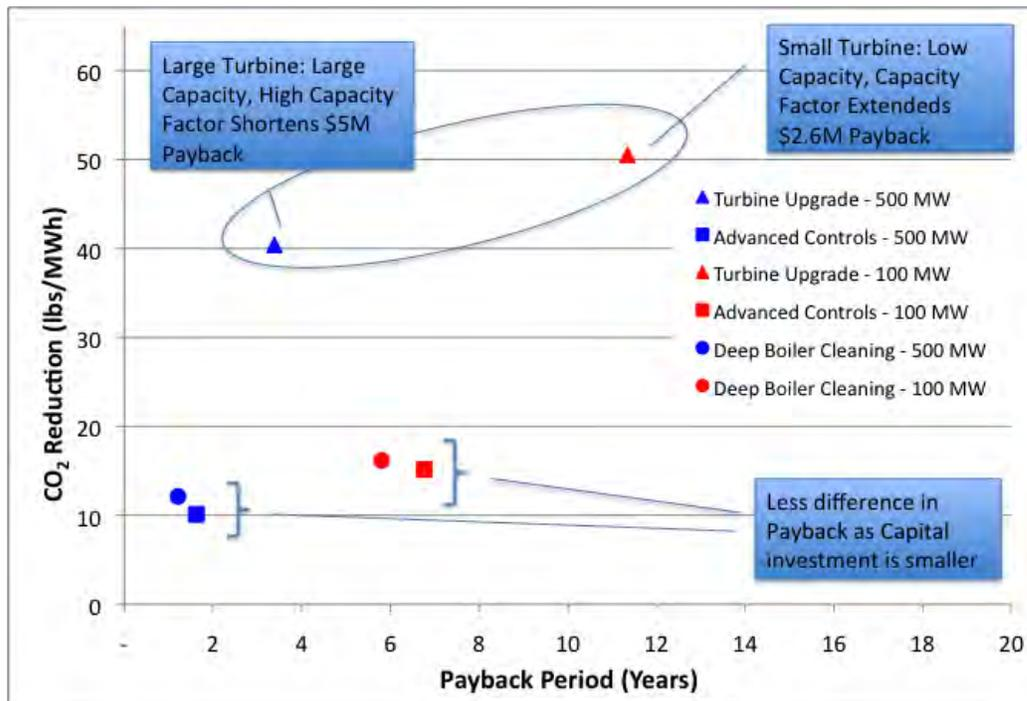
Figure 5-2. CO2 Reduction vs. Calculated Payback Period
