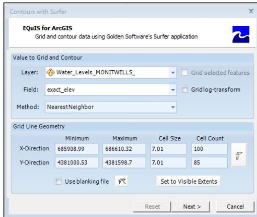
Figure 27 – Setting the Layer, Field and Method for Contours with Surfer
