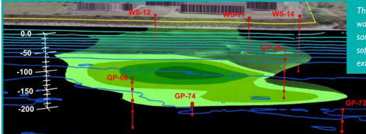
The use of electronic ground water and surface water sampling data in visualization software can help illustrate the extent of a contaminant plume.
