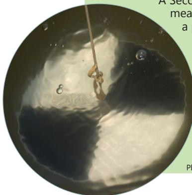
A Secchi disk is used to measure how deep a person can see into the water, and provides an approximate evaluation of the transparency of water.
