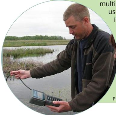
Water quality multiprobes are often used to collect data in the field on temperature, dissolved oxygen, conductivity, pH, and other parameters.
