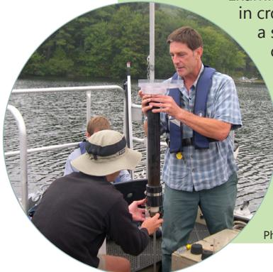
Examination of diatoms in cross sections of a sediment core can provide insight on a lake's historical chemical and physical characteristics, such as total phosphorus and clarity.
