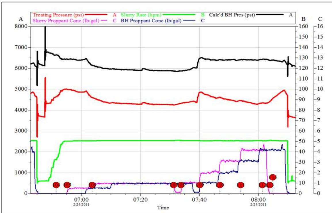
Figure 8 Treatment Chart -- Pressure, Rate and Prop Concentration
