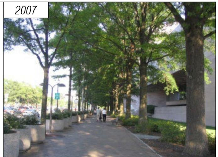
Above: Trees on the left side of this sidewalk were planted with significantly smaller root growth area vs. the right. Even after almost 30 years, these trees still show a significant size differential. Trees along the street have roughly 300 cubic feet of growth area vs. the right with large green space. Pennsylvania Avenue Northwest, Washington, DC. (Casey Trees, 2008)
