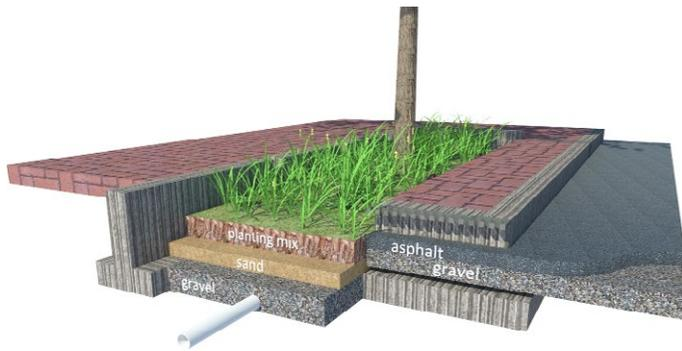
Treated stormwater is then either infiltrated into the ground as groundwater (infiltration planters) or discharged into a conventional storm sewer pipe (flow-through planters), where infiltration is not appropriate.
