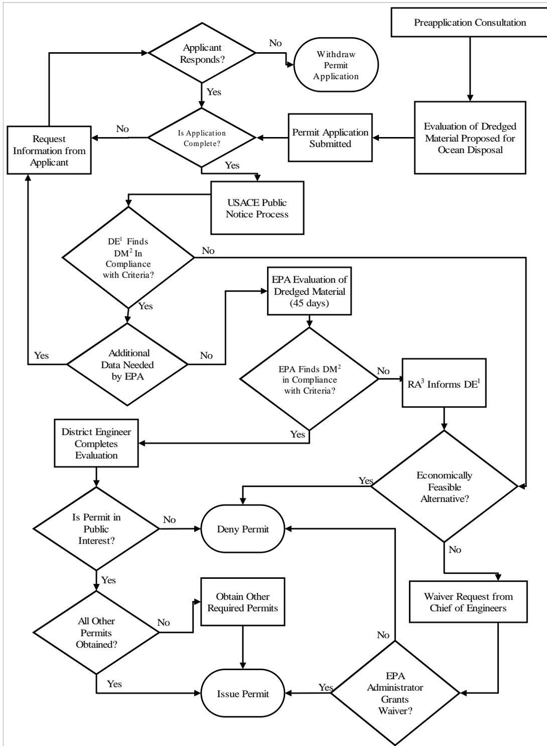
**Figure 2: Permit Application/Evaluation Procedure**
