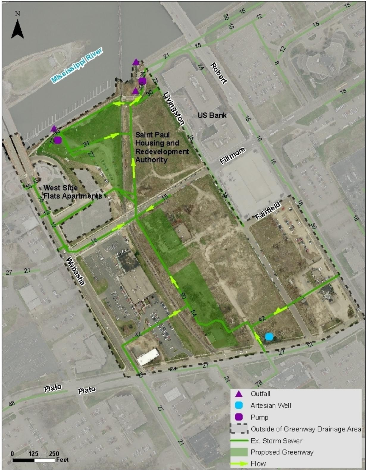
Figure 3. Greenway Drainage Area Site Conditions
