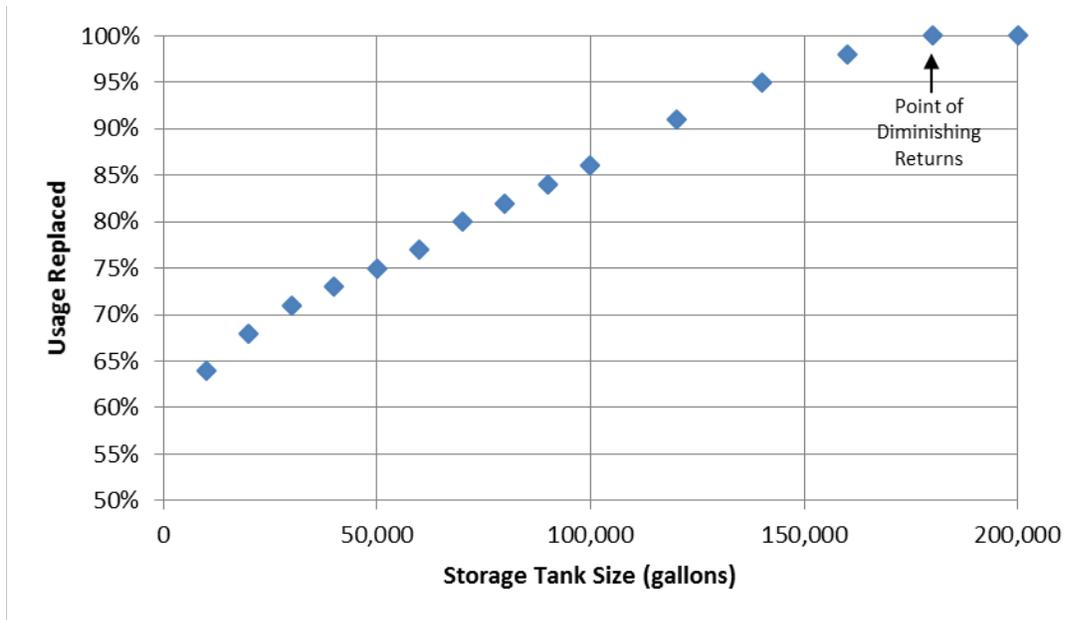
Figure 4-5. Wet-weather cistern sizing versus potable supply offset for Ozone Park.
