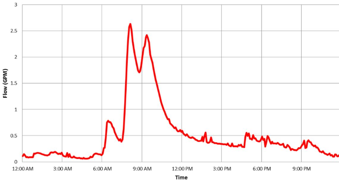
Figure 4-2. Typical dry-weather flow 24-hour distribution for Ozone Park.
