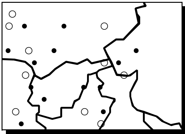
Figure 3-1b. Simple random sampling from a map. Dots represent sites. All sites of interest are represented on the map, and the sites to be sampled (open dots—○) were selected randomly from all of those on the map. The shaded lines on the map could represent county, watershed, hydrologic, or some other boundary, but they are ignored for the purposes of simple random sampling.
