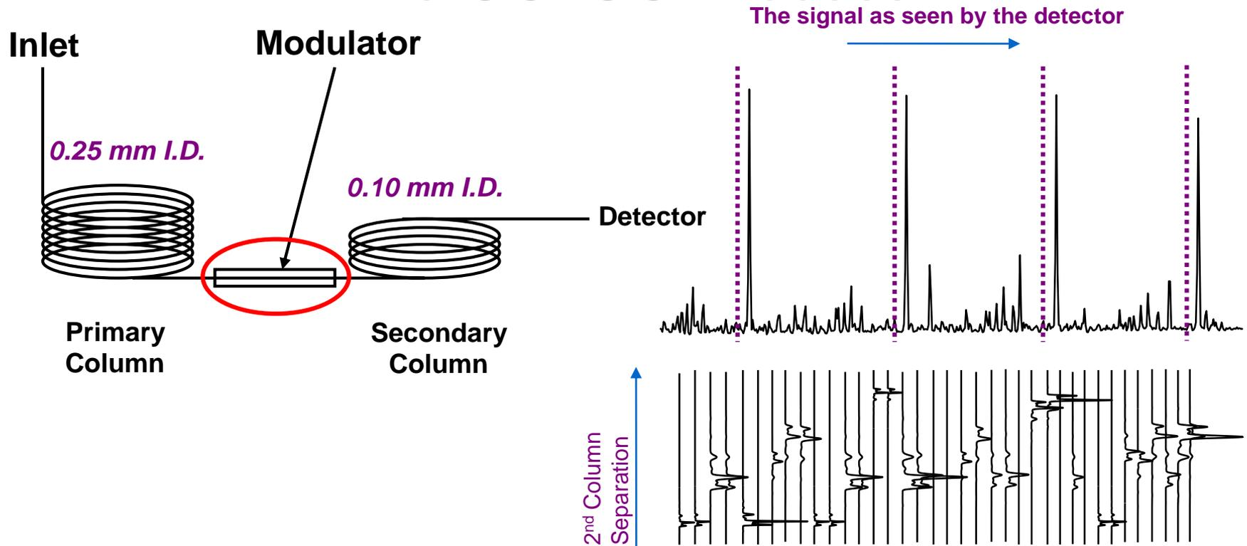
The effluent from the primary column is focused and segmented by the modulator into a discrete "plug". Each plug is then injected onto the secondary column by the modulator, where it is separated. The GCxGC process is a series of independent second column separations.
