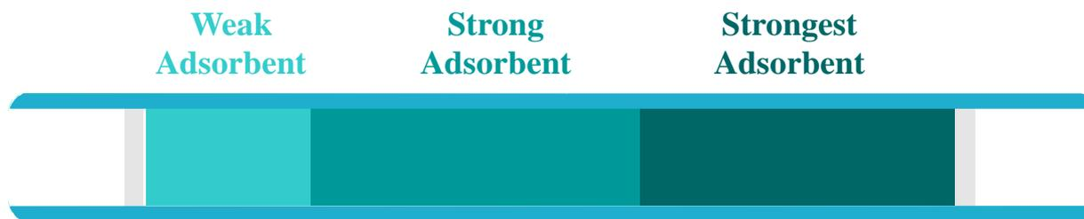
Sample the tube in the direction of weak adsorbent to strong adsorbent
