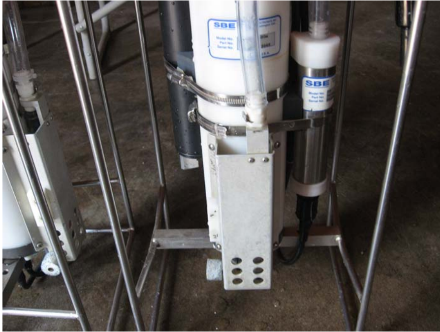
Figure 3-1. Sea-Bird SBE-19 CTD Sensor with Integrated SCUFA® Fluorometer
