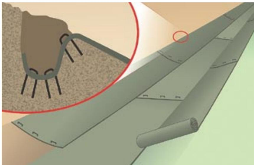
*Lay in ditch blankets similar to roof shingles; start at the lowest part of the ditch, then work your way up. Uphill pieces lap over downhill sections. Staple through both layers around edges. Trench, tuck, and tamp down ends at the top of the slope. Do not stretch blankets or mats.*
