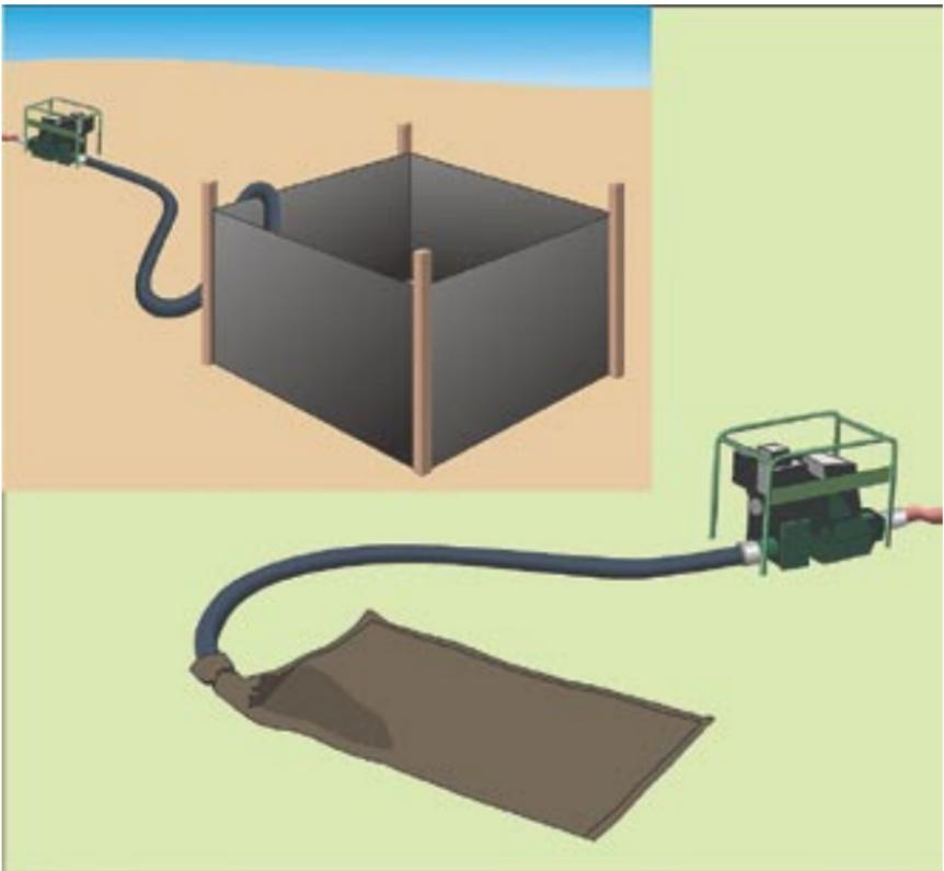
*Pump muddy water from dewatering operations away from waterways into a silt fence enclosure or use a bag filter or other device to remove sediment. Allow discharge to soak into the ground if possible. Do not pump discharger from dewatering operations into curb inlets, storm sewers, creeks, lakes, or rivers without a KPDES permit from the Division of Water.*
