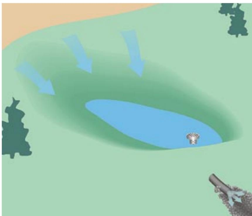
*Sediment basins often have pipe risers, but well-constructed rock overflow outlet notches in the dam or retaining berm are acceptable if the overflow area is protected from erosion.*
