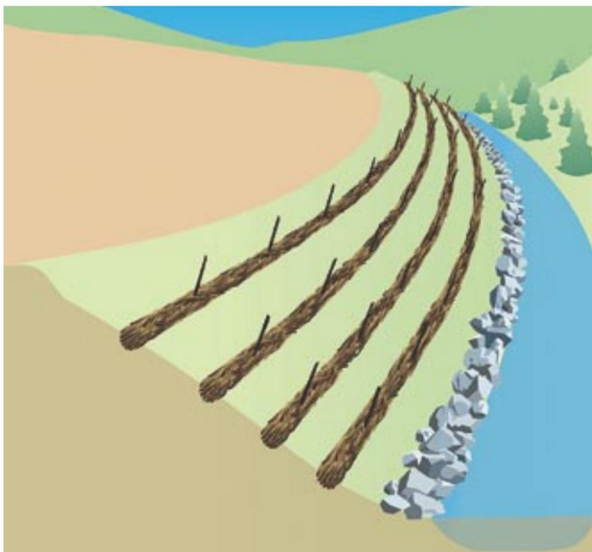
*Live willow or hardwood stakes driven through live wattles or rolls, trenched into slope, provide excellent stream bank protection. Protect toe of slope with rock or additional rolls or wattles.*
