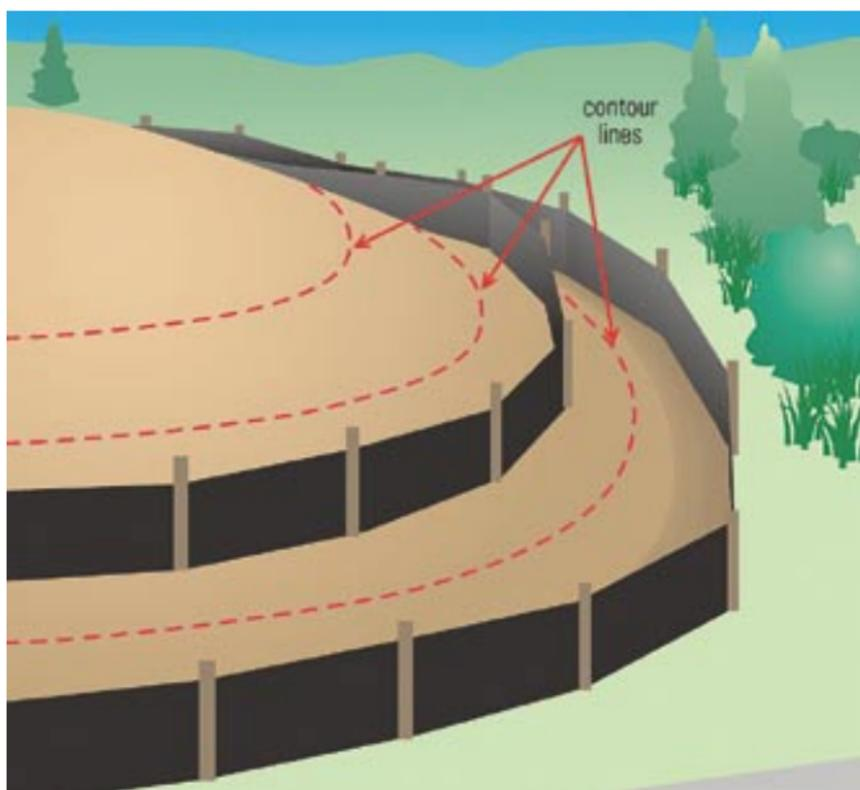
*Silt fences should be installed on the contour below bare soil areas. Use multiple fences on long slopes 60 to 80 feet apart. Remove accumulated sediment before it reaches halfway up the fence.*
