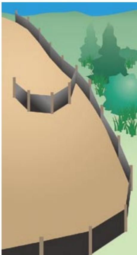
*Use J-hooks to trap and pond muddy runoff flowing along uphill side of silt fence. Turn ends of silt fence toward the uphill side to prevent bypassing. Use multiple J-hooks every 50 to 150 feet for heavier flows.*
