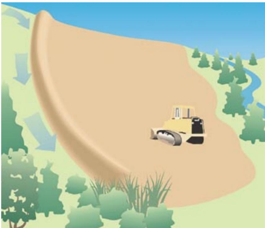
*Berms and ditches diverting clean upland runoff around construction sites reduce erosion and sedimentation problems. Seed berms and ditches after construction.*
