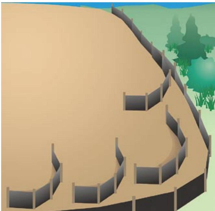
*Silt fences don't have to be on the property line. Placing them on slopes with the ends turned up to trap sheet flow provides better performance. Stagger fence sections to ensure total coverage. Clean out before sediment reaches halfway up. Repair as needed, and remove when grass is well established.*
