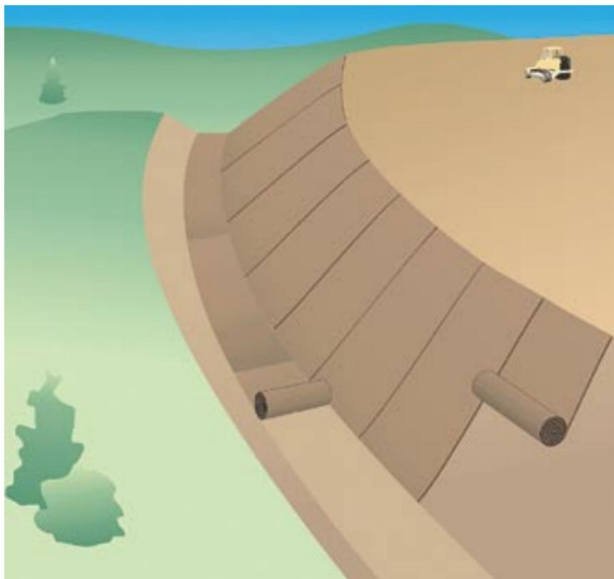
*Steep, long slopes need blankets or mats. Install blankets and mats up and down long slopes. For channels below slopes, install horizontally. Don't forget to apply seed, lime, and fertilizer (if used) before installing blanket.*
