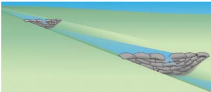
Silt check dams of rock, stone-filled bags, or commercial products must be installed before uphill excavation or fill activities begin. See table for correct silt check spacing for various channel slopes. Tied end of bag goes on downstream side.
