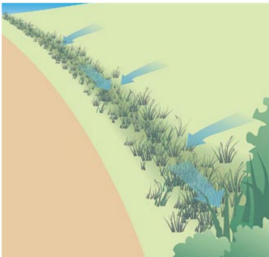
*Diversion ditches should be lined with grass at a minimum, and blankets if slopes exceed 10:1 (10%) (see Section 8).*
