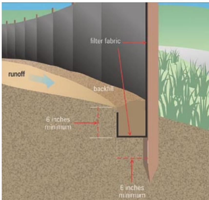
*Remember: stakes go on the downhill side. Dig trench first, install fence in downhill side of trench, tuck fabric into trench, then backfill on the uphill side (the side toward the bare soil area).*
