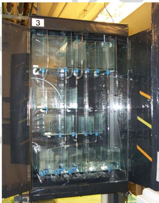
**Figure 2.2.** Continuous-flow proportional diluter system
