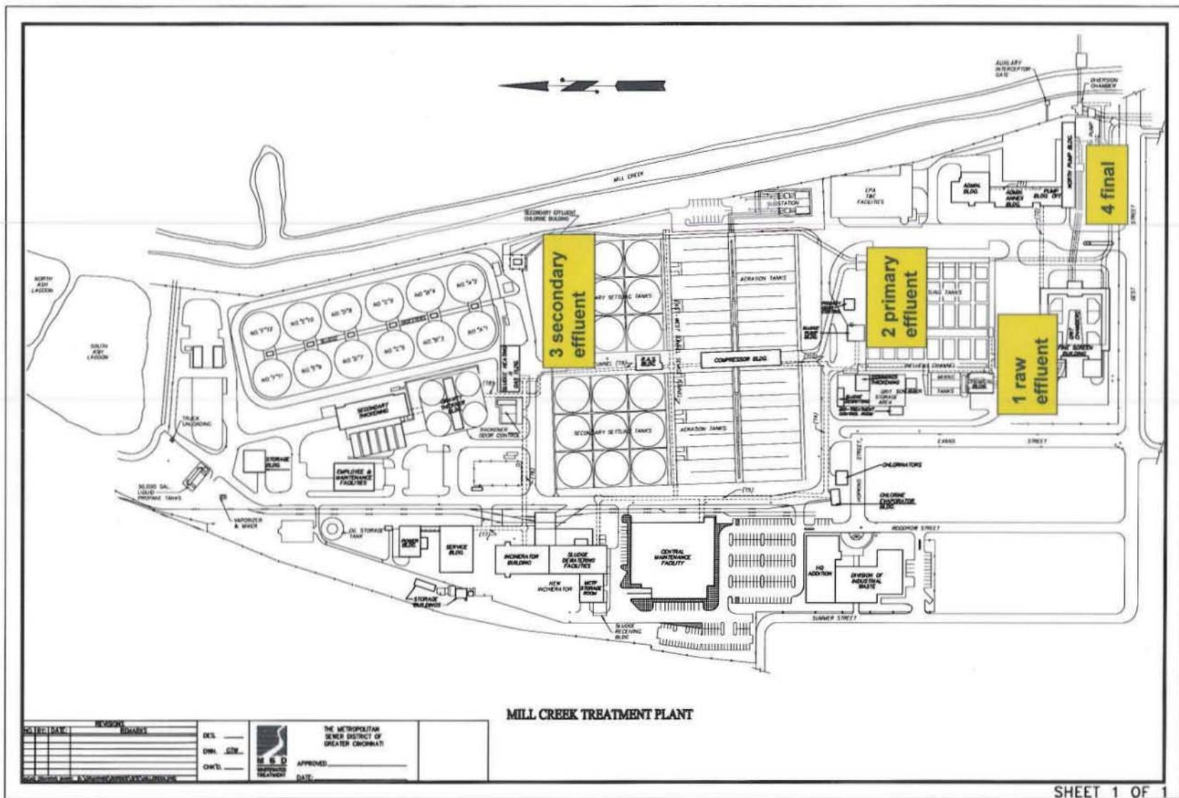
Fig. A1. Schematic of Mill Creek WTP, an activated sludge treatment plant in Cincinnati, Ohio that uses chlorination.
