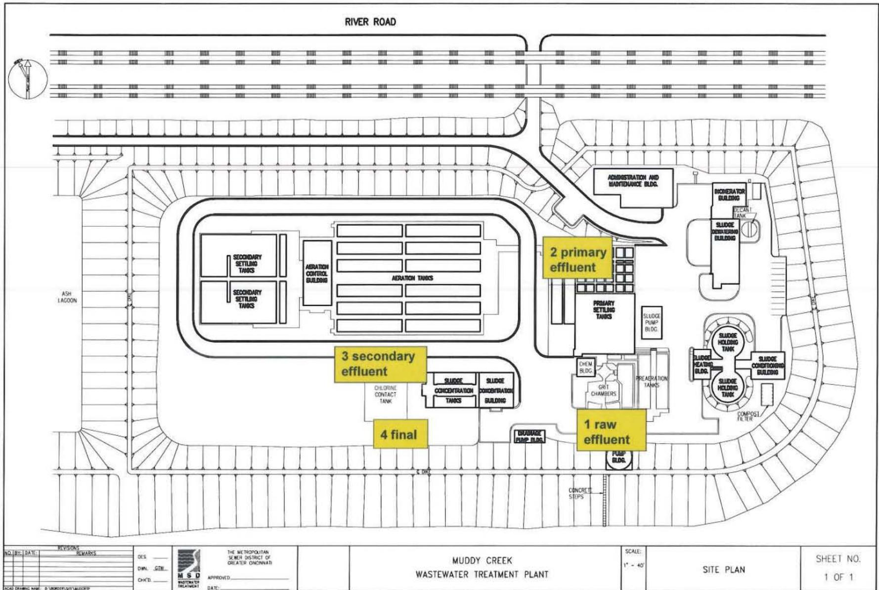
Fig. A2. Schematic of Muddy Creek WTP, an activated sludge treatment plant in Cincinnati, Ohio that uses ultraviolet light disinfection.
