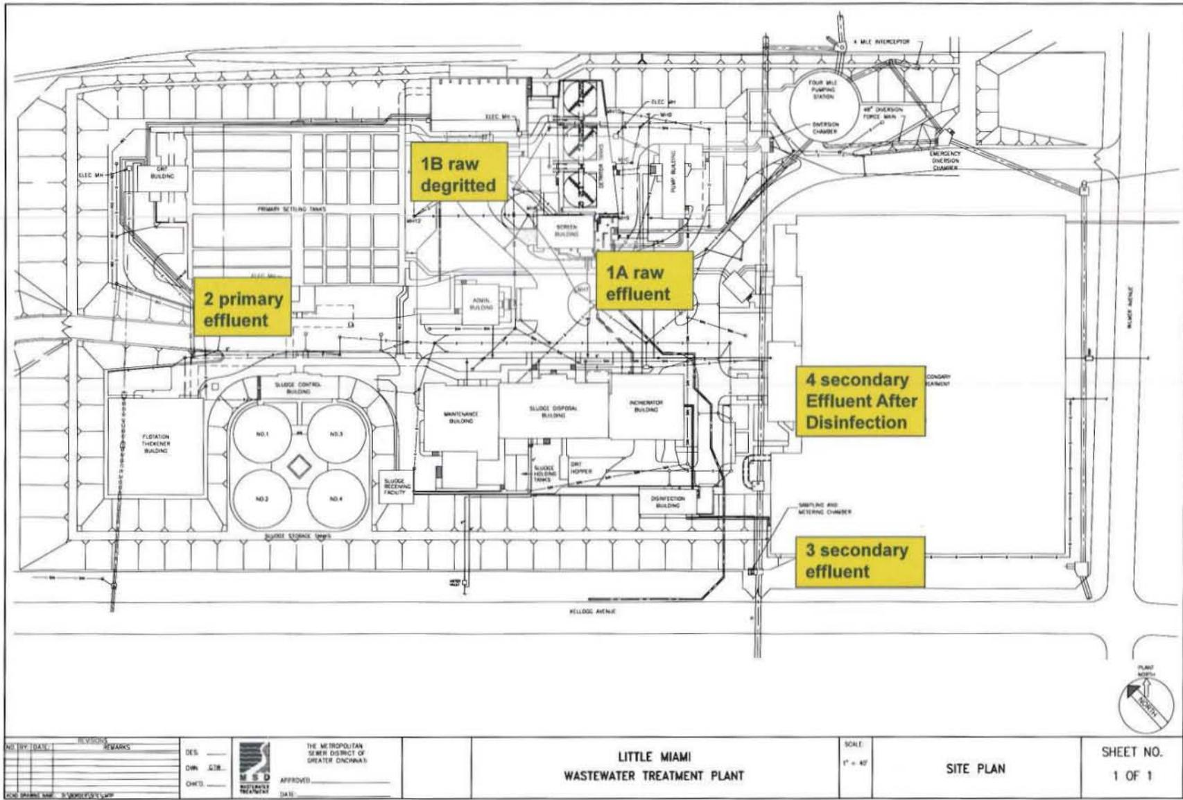
Fig. A3. Schematic of Little Miami WTP, an activated sludge treatment plant in Cincinnati, Ohio that uses chlorination.
