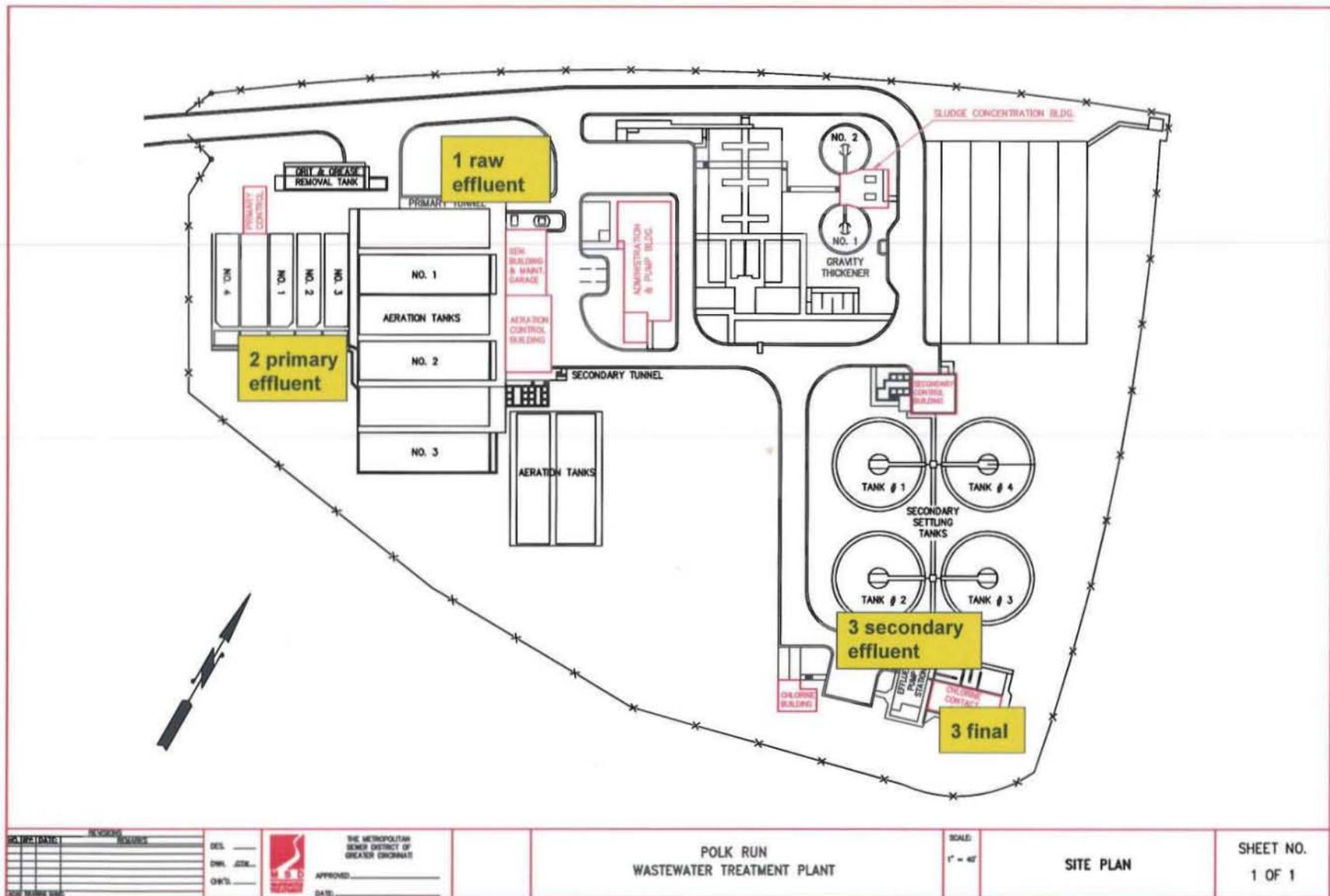
Fig. A4. Schematic of Polk Run WTP, an activated sludge treatment plant in Cincinnati, Ohio that uses ultraviolet light disinfection.
