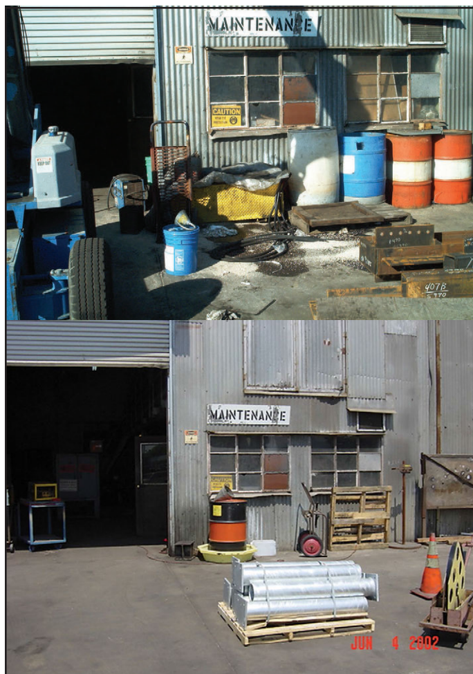
Figure 6. Two photos showing an industrial facility before and after it followed good housekeeping practices.
