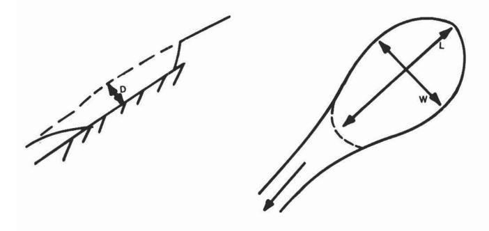
Figure V.9.—Dimensions of debris avalanche-debris flow failures for determining potential volumes. W = width; L = length; D = depth.
