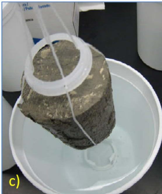
c) Removing Sample for Exchange
