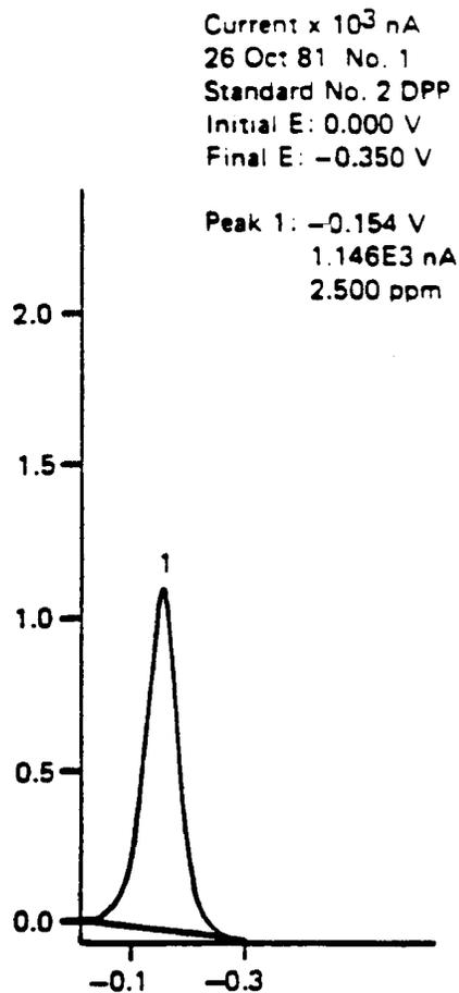
Figure 2. Typical differential pulse polarogram at 0.25 ppm and 2.5 ppm Cr in 0.1 N buffer.
