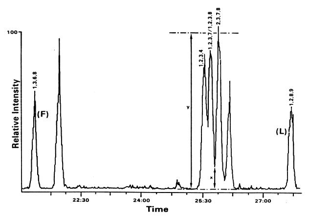
Selected ion current profile for m/z 322 (TCDD) produced by MS analysis of GC performance check solution on a 60 m x 0.32 mm DB-5 fused silica capillary column with 0.25  $\mu$ m film thickness.
