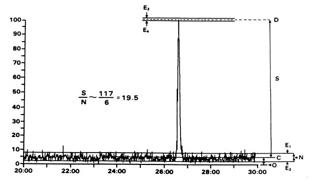
The peak height (S) is measured between the mean noise (lines C and D). These mean signal values are obtained by tracing the line between the baseline average noise extremes, E1 and E2, and between the apex average noise extremes, E3 and E4, at the apex of the signal.
