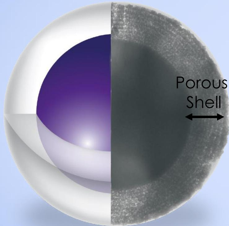
**Monodispersed silica particles consisting of an impermeable silica core surrounded by a layer of fully porous silica**
