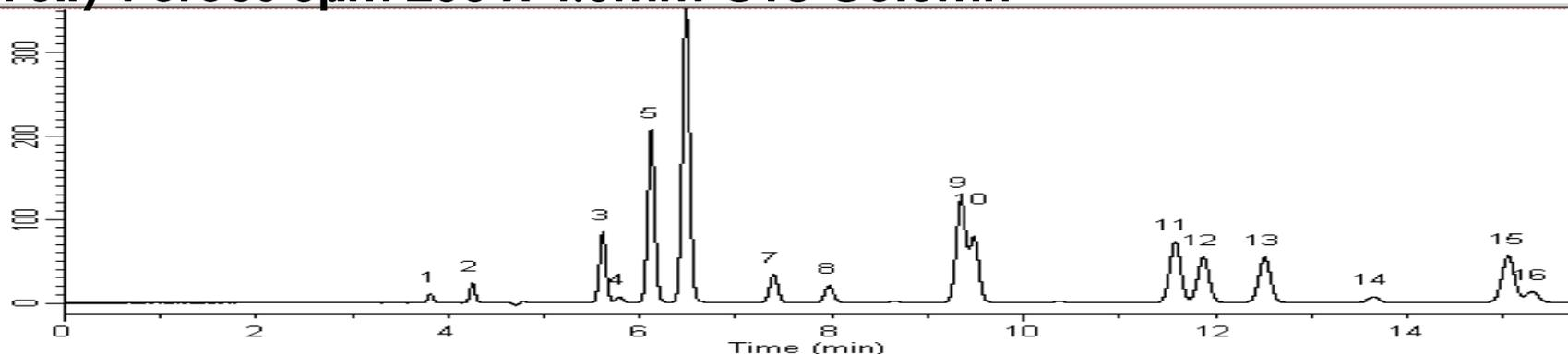
**Kinetex® 2.6 $\mu$ m 100 x 4.6mm C18 Column**
