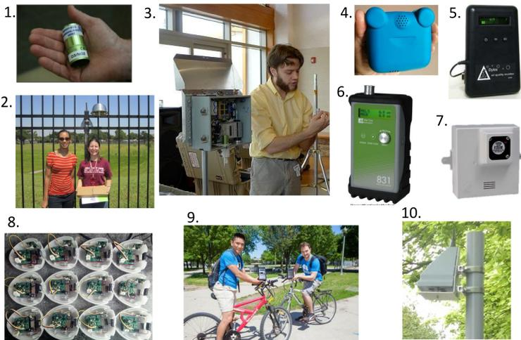
*Notes:* 1. Cairpol nitrogen dioxide/ozone sensor; 2. School application of nitrogen dioxide sensor during DISCOVER-AQ study; 3. Citizen Science Air Monitor (CSAM) demonstration; 4. AirBeam particle sensor developed by HabitatMap's AirCasting project; 5. Dylos particle counter; 6. MetOne particle counter; 7. Shinyei particle sensor; 8. Air Quality Eggs; 9. Community group operating Dylos particle counters on bicycles; 10. AQMesh multipollutant sensor system.
