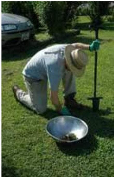
*Taking a soil sample is a simple and routine process. This investigator is seen using a hand auger to dig a small hole in the soil that can then be placed in the bowl for laboratory analysis.*
