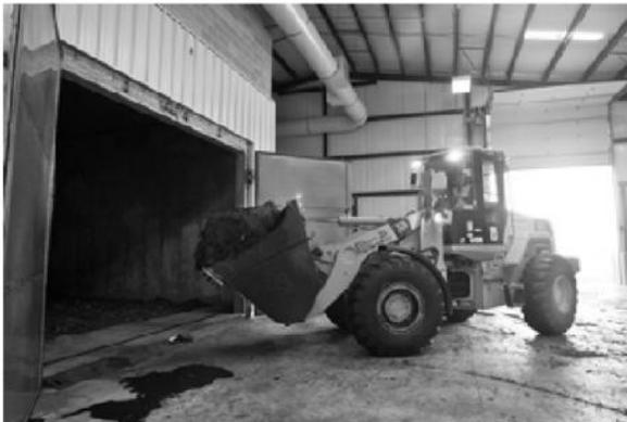
A front-end loader delivers compostable material into one of the chambers of the UW Oshkosh Biodigester, first of its kind in the western hemisphere.
