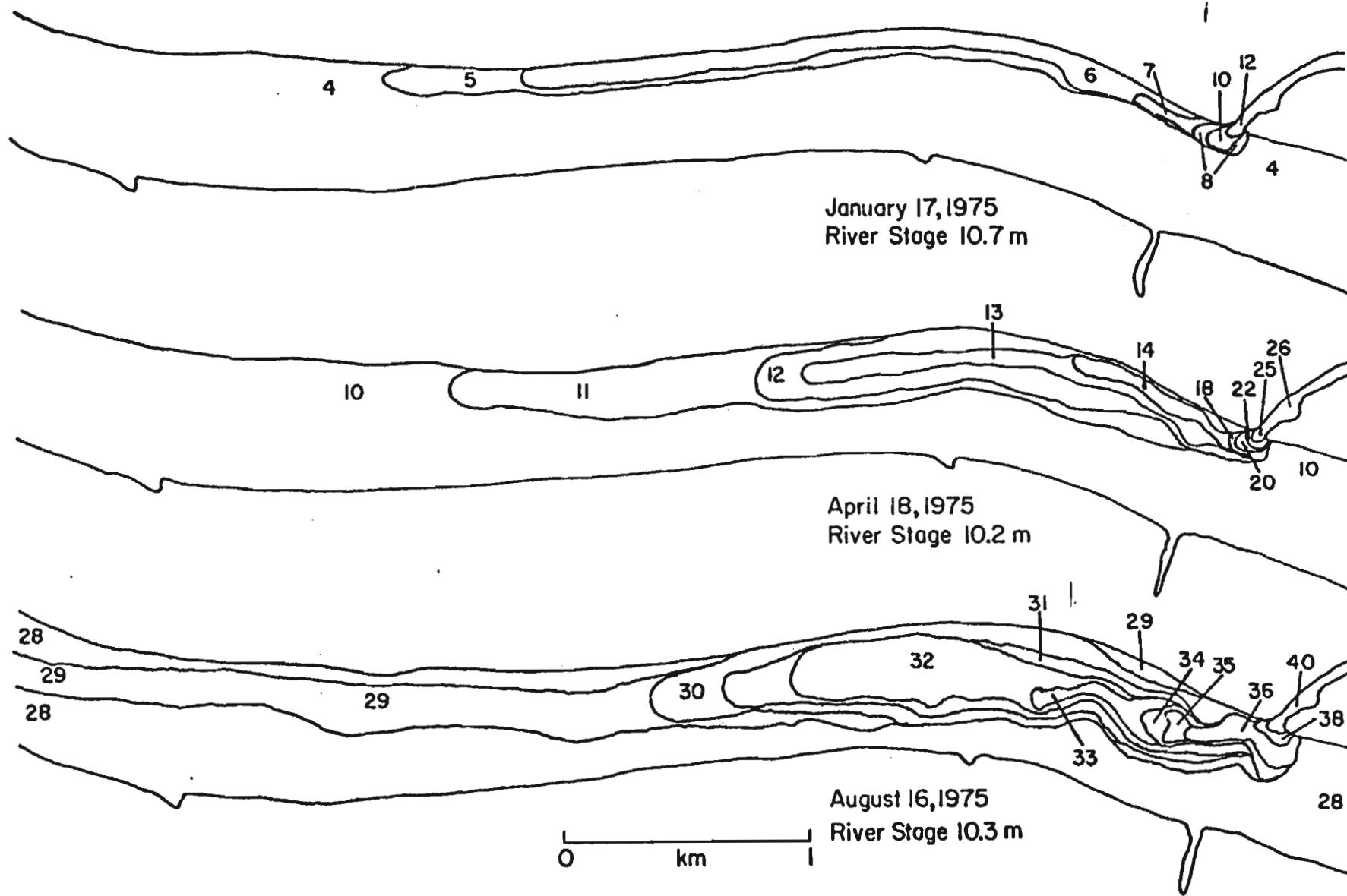
FIGURE V-16 Thermal plume configuration in °C downriver from the J. M. Stuart discharge canal during January, April, and August 1975 (from Yoder and Gammon, 1976).
