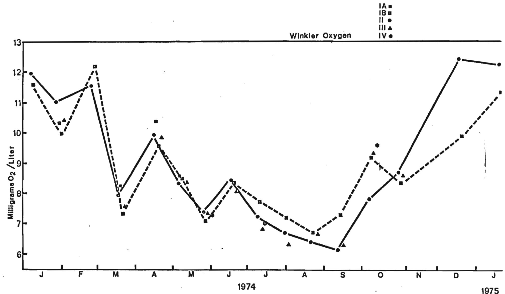
FIGURE VI-2      Dissolved oxygen concentration determinations at the J. M. Stuart Station
