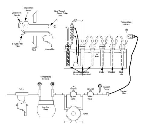
Figure 207-1-1. Sampling Train Configuration for Isocyanates
