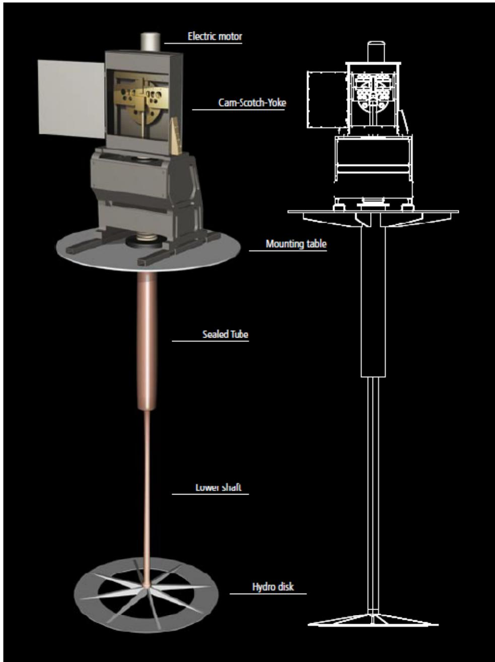
Figure 7-1 Vertical Linear Motion Mixer by Enersave Fluid Mixers, Inc.
