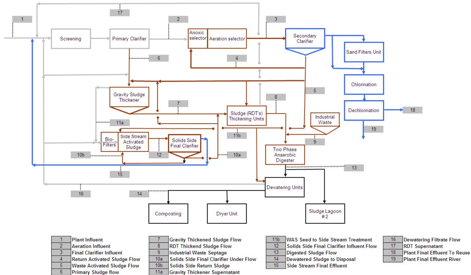
**Figure 2: WMARSS Process Flow Diagram**
