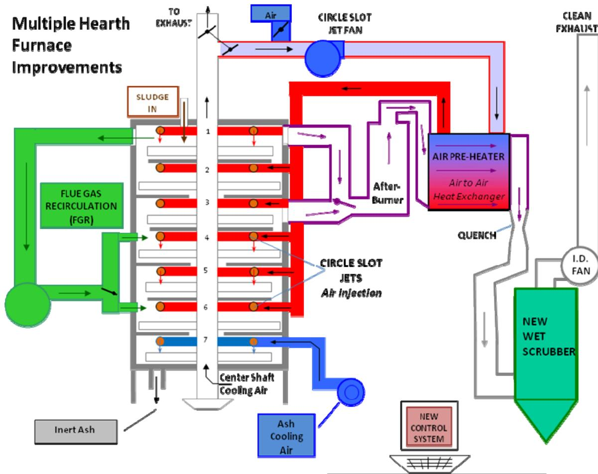
**Figure 3: Schematic of MHF Improvements at the Western Branch WWTP**
