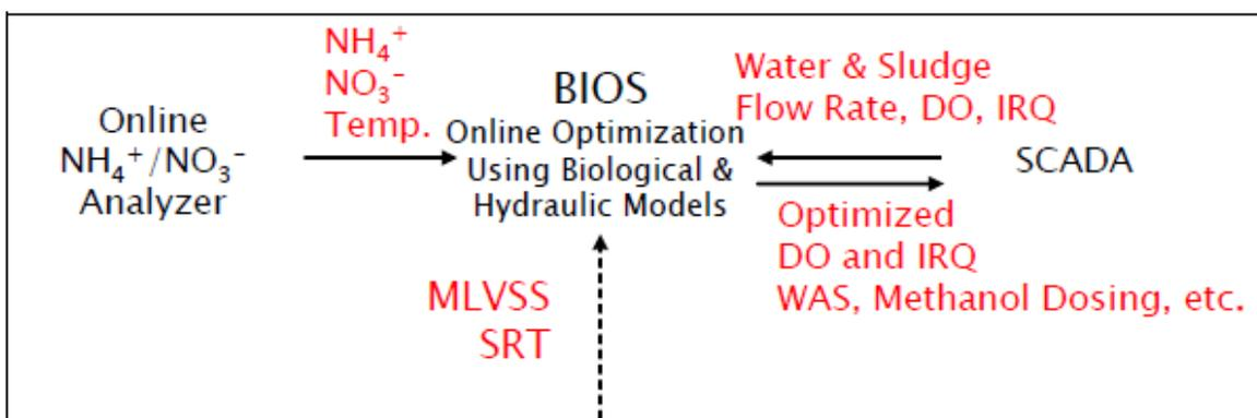
Figure 4-6. Representation of the BIOS process
