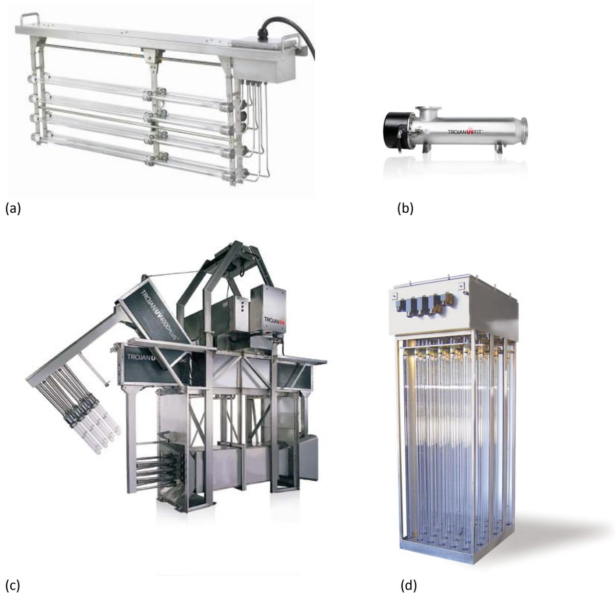
Figure 6-1. Example UV Lamp Configurations for Wastewater Treatment (a) Calgon C<sup>3</sup>150 for open channel flow, horizontal and parallel lamp arrangement (b) TrojanUVFit for closed channel flow (c) TrojanUV4000Plus for open channel flow, horizontal and parallel lamp arrangement, and (d) Aquaray® 3X Vertical Lamp System for open channel flow, perpendicular lamp arrangement. Used with permission.
