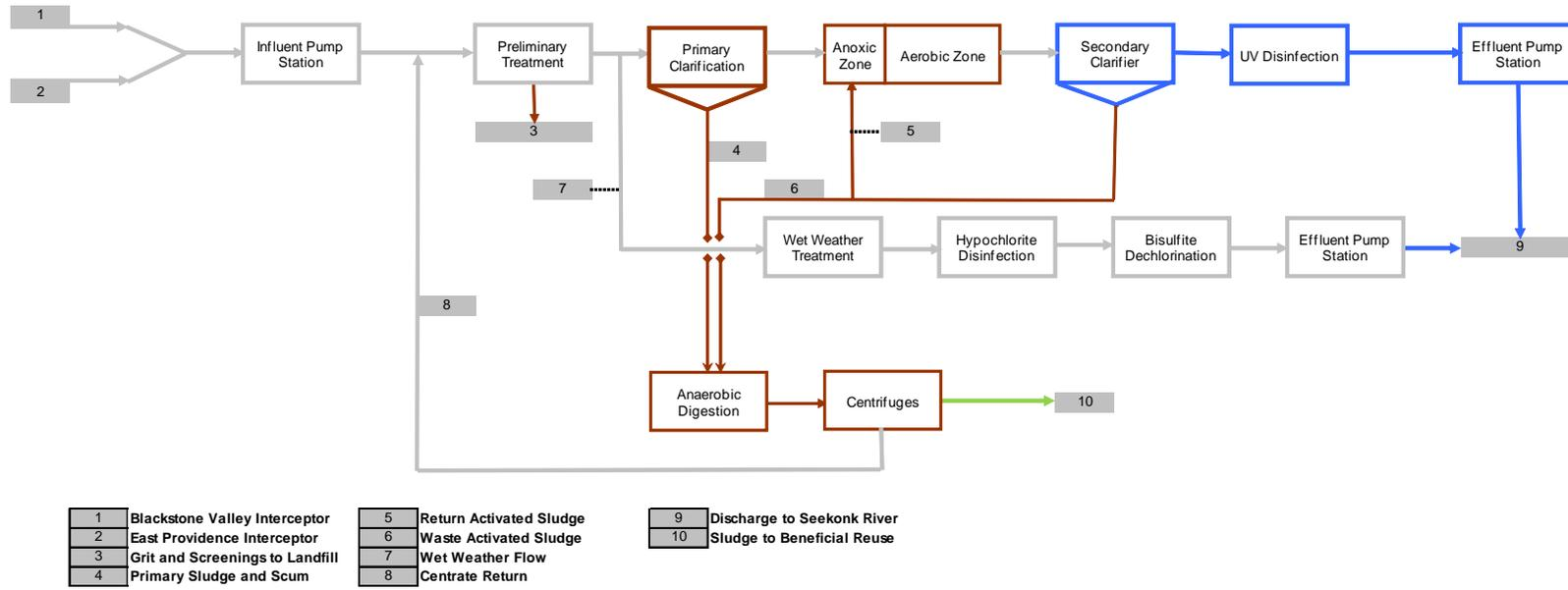
**Figure 2: NBC Bucklin Point WWTF Process Flow Diagram**
