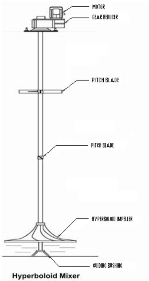
Figure 6-2. Typical Installation of a Hyperboloid Mixer
