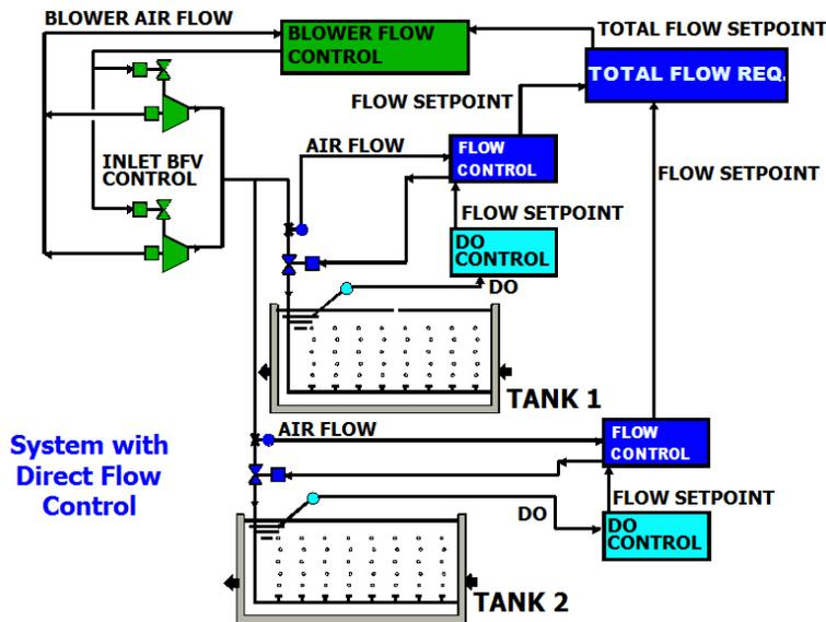
Figure 4-4 Integrated Air Flow Control System for Automated DO Control
