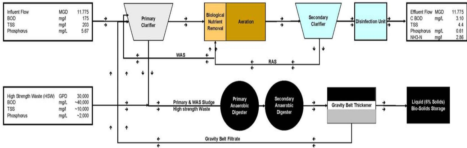
**Figure 2: Sheboygan Wastewater Treatment Plant Process Flow Diagram**
