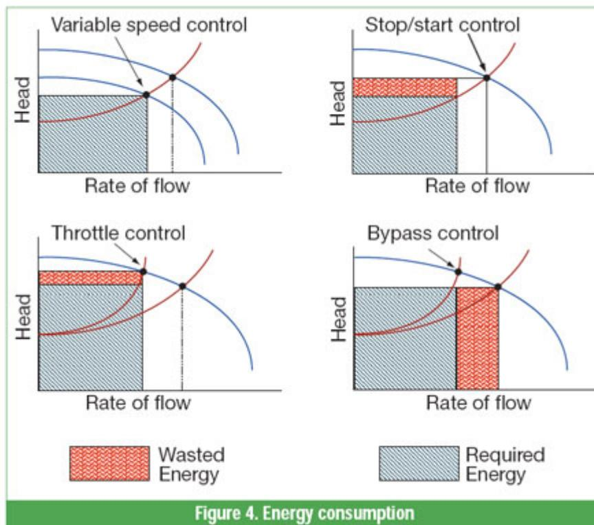
Figure 3-2. Wasted Energy in Alternative Control Schemes Compared to Variable Frequency Drives
