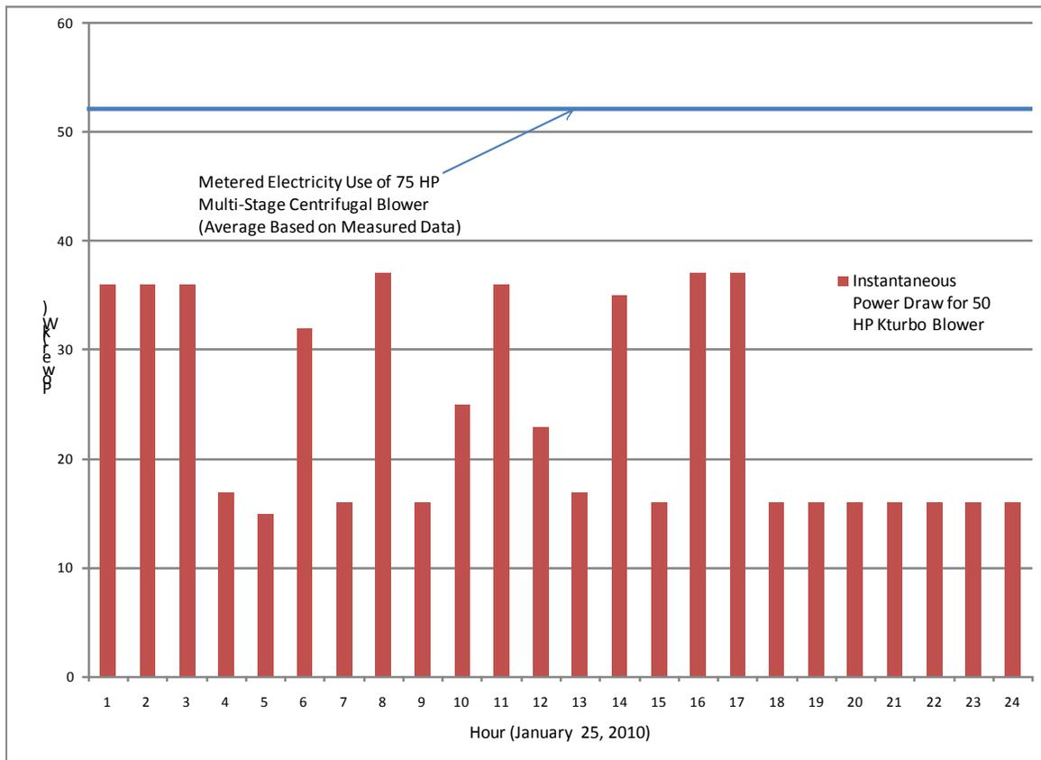
Figure 5-3. Comparison of Power Draw for Old and New Blower at Burlington, VT
