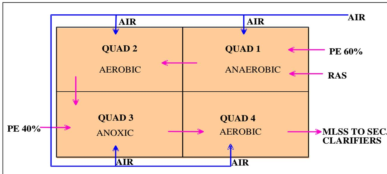
Figure 3: SJ/SC WPCP BNR Process Flow Diagram
