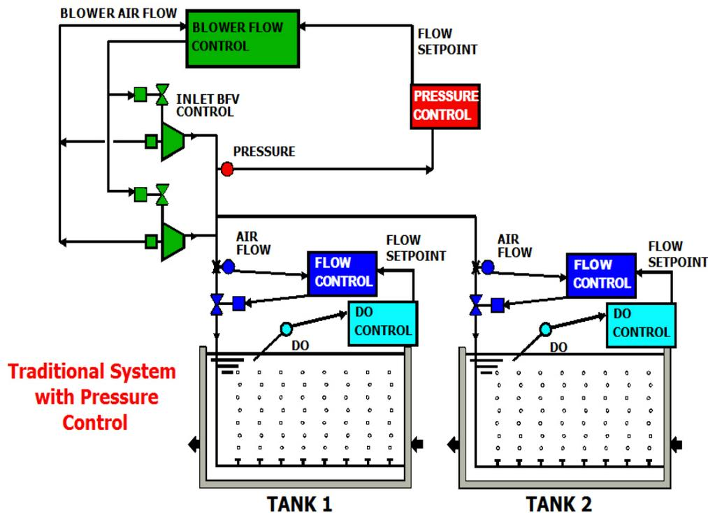
Figure 4-2 Common Cascade System for Automated DO Control
