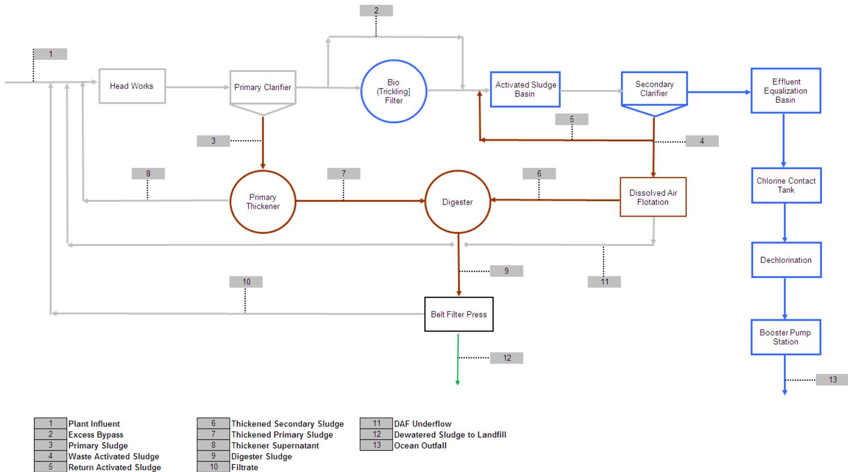
**Figure 2: Oxnard WWTP Process Flow Diagram**
