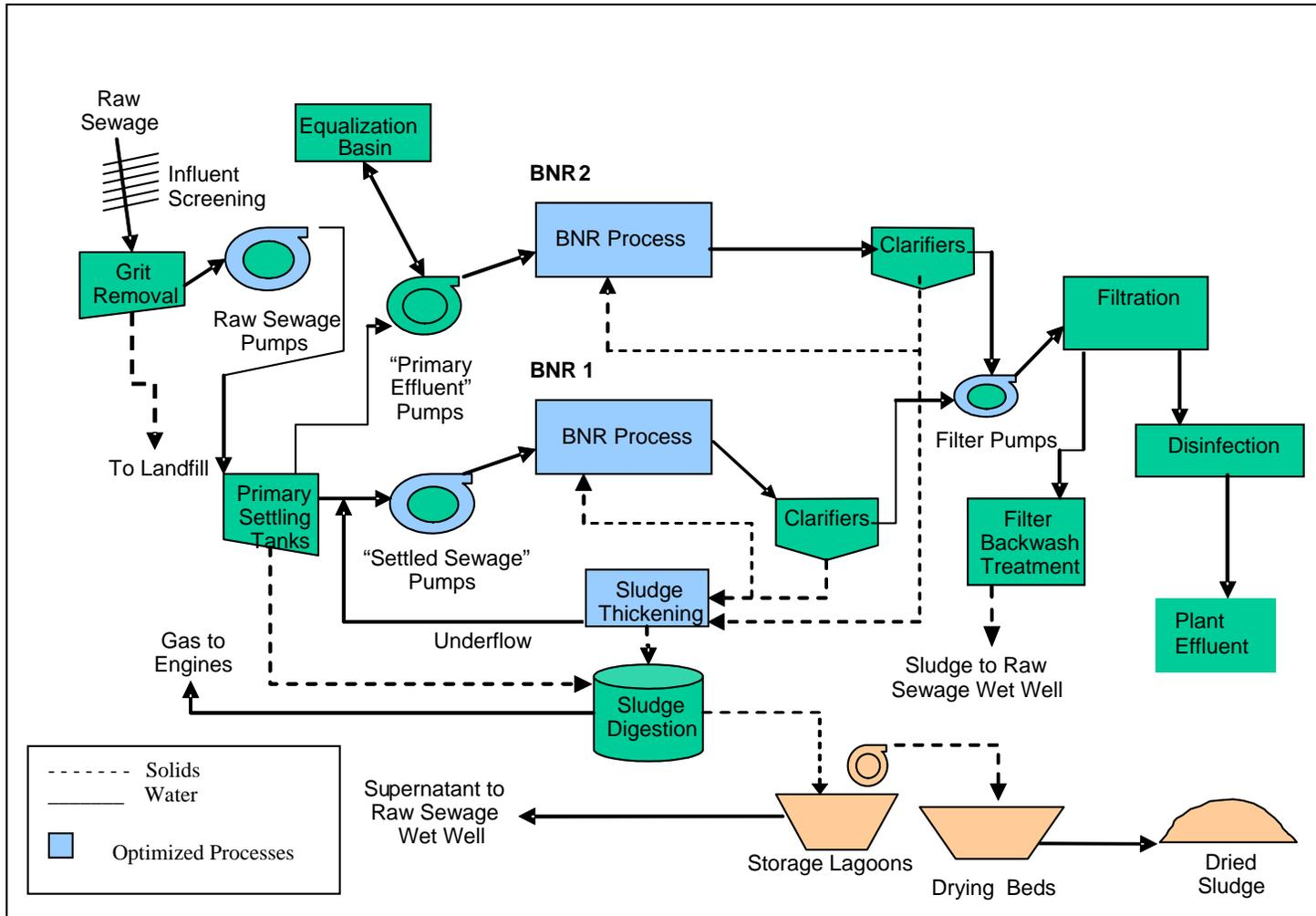
**Figure 2: SJ/SC WPCP Treatment Process Flow Diagram**
