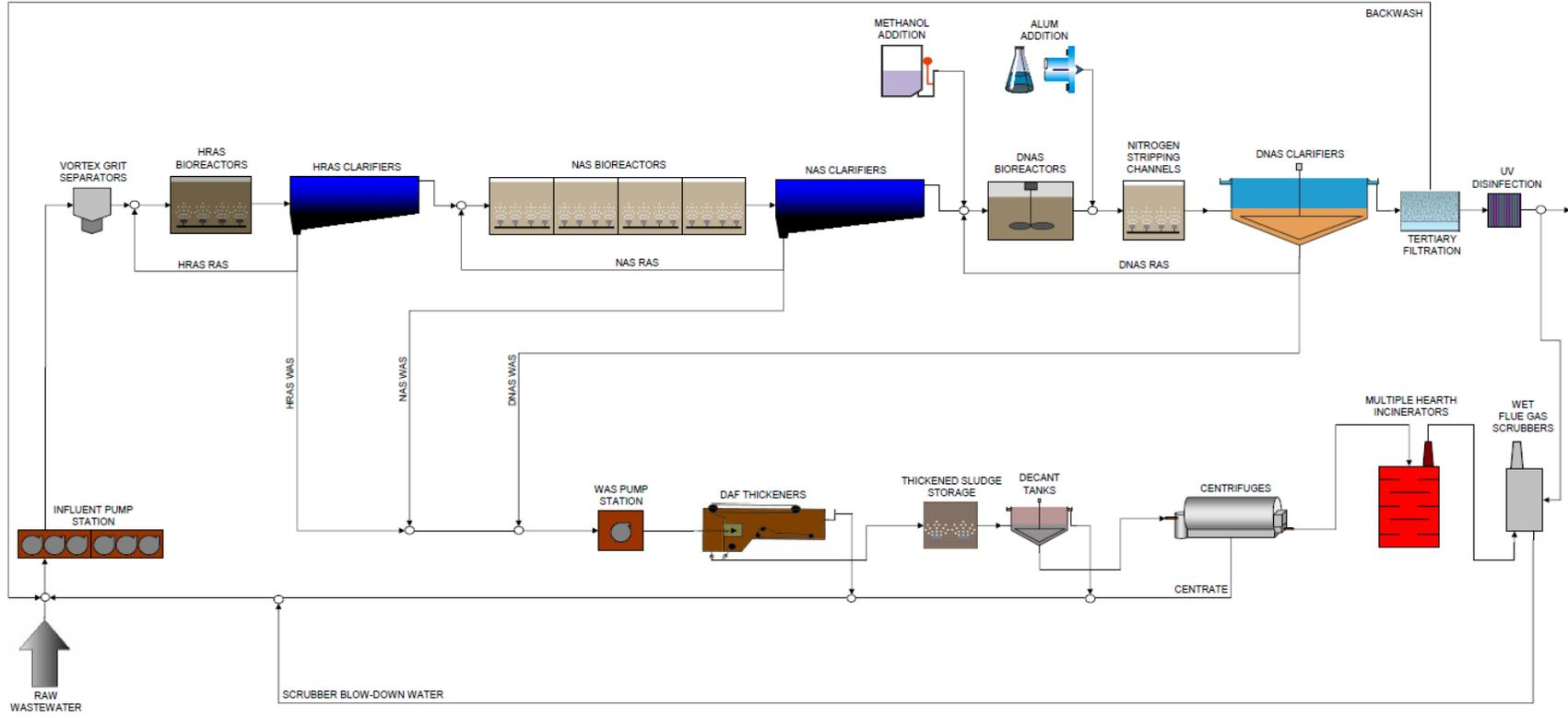
**Figure 2: WSSC Western Branch WWTP Process Flow Diagram**
