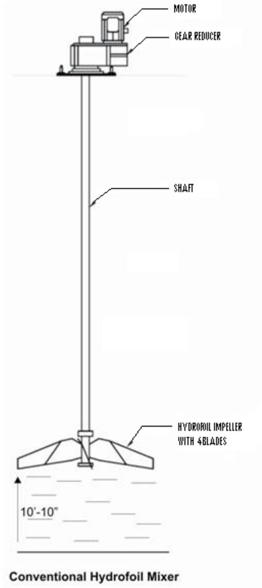
Figure 6-3. Conventional Hydrofoil Mixer
