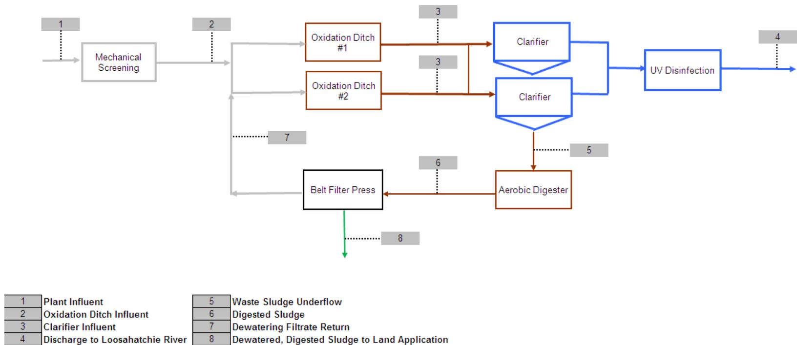
**Figure 3: City of Bartlett WWTP #1 Process Flow Diagram**
