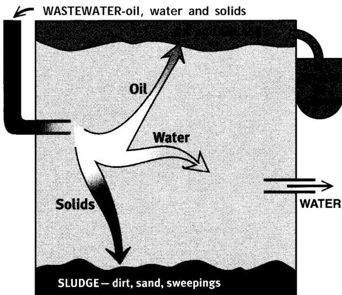
*Heavier or Lighter Than Water?* OWSs treat vehicle and floor wash water by allowing substances lighter than water to float and substances heavier than water to sink. Many OWSs also have baffles, coalescers, and oil skimmers to speed-up or enhance separation of these substances.
