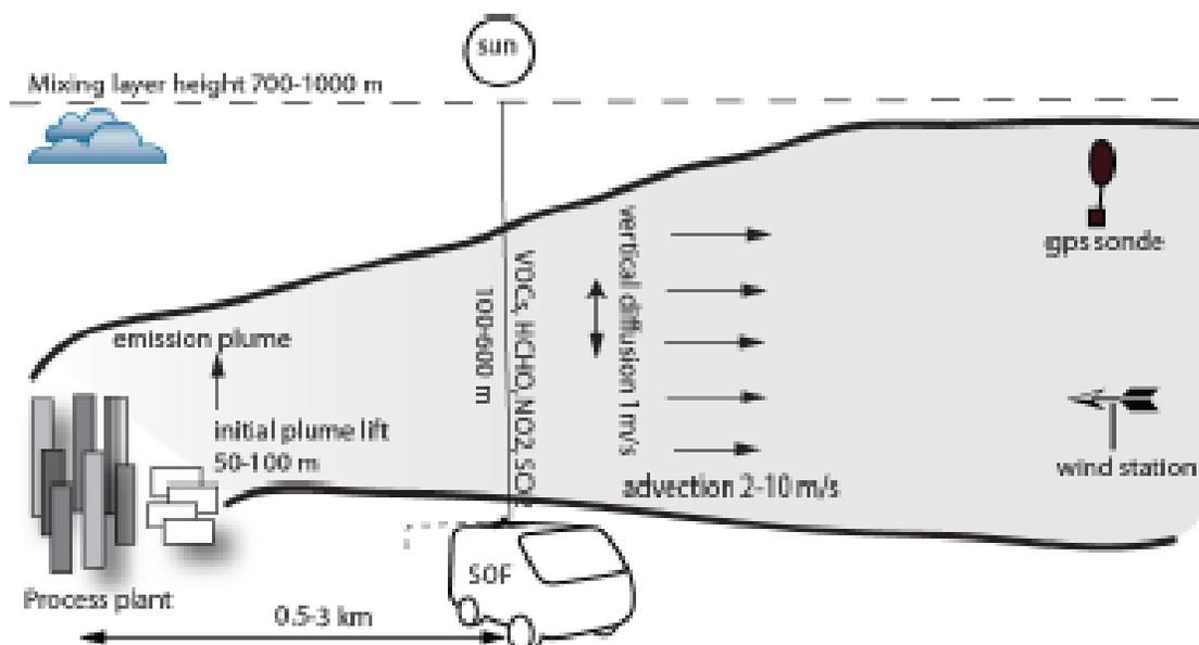
**Figure 2-4. Schematic of SOF measurement technique. Figure from Johansson et al. (2012).**
