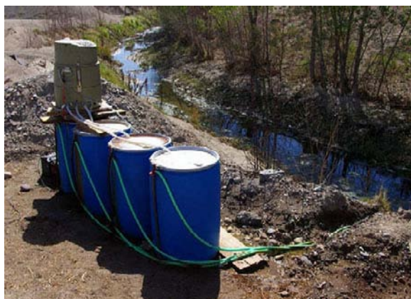
Selenium bench-scale bioreactors funded by the U.S. Bureau of Reclamation are being tested to determine their ability to reduce selenium concentrations in 303(d) listed tributaries of the Grand Valley and Gunnison Basin. Photo by Dr. Russ Walker, Mesa State College, Colorado.
