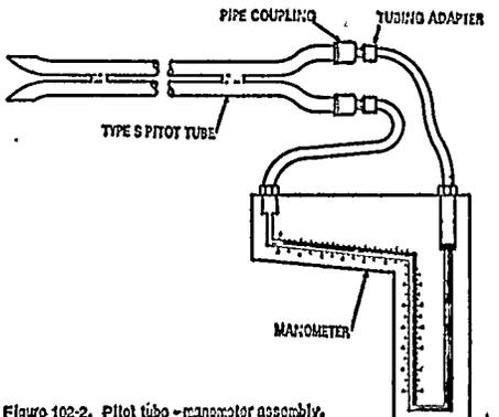
Figure 102-2. Pitot tube-manometer assembly.
