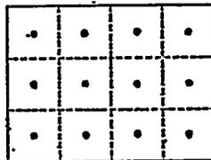
Figure 104-5. Cross section of rectangular stack divided into 12 equal areas, with traverse points at center of each area.
