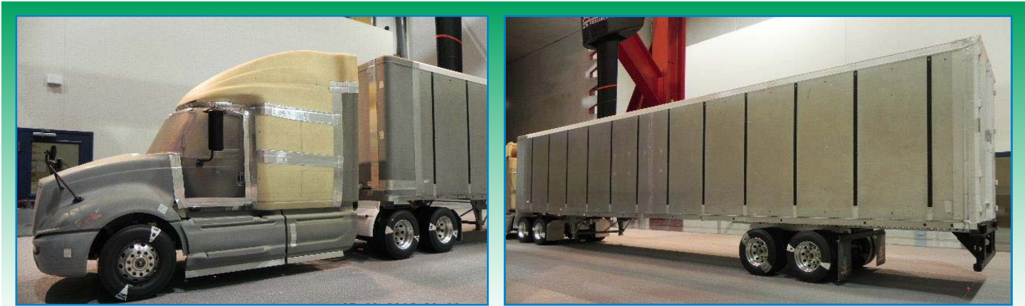
Testing at Auto Research Center's (ARC's) 1/8th scale wind tunnel using a model tractor and box trailer
