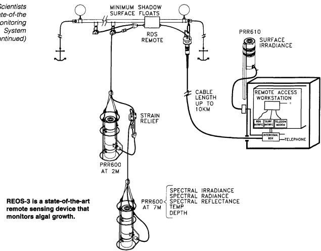
The REOS-3 system works by monitoring algal biomass with a pair of reflectance radiometers that are permanently submerged in the reservoir. The radiometers, which were developed by BSI to provide ground truth for NASA ocean color satellites, measure both the natural fluorescence of planktonic algae and the attenuation of ambient light passing through the water column. These independent measurements support estimates of the algal standing crop.
