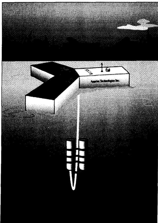
**RUSS is equipped with an on-board computer powered operated by remote control through cellular phone transmission. A device attached to a multiprobe sensor moves up and down the water column, sampling pH, conductivity, turbidity, dissolved oxygen, and temperature at depths up to 100 meters.**
