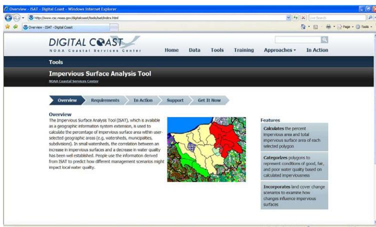
The first page of the Impervious Surface Analysis Tool (ISAT) provides a road map for using the tool, including tabs with overview information, the technical and data requirements for using ISAT, examples of ISAT in action, online ISAT help and tutorials, and how to download ISAT.
