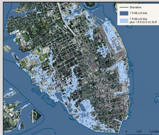
**An assessment of Charleston, South Carolina shows the amount of inundation that would occur with both a 7-foot mean lower low water (MLLW) tide—the observed average of the lower low water height of each tidal day—plus an 18-inch sea level rise (SLR).**
