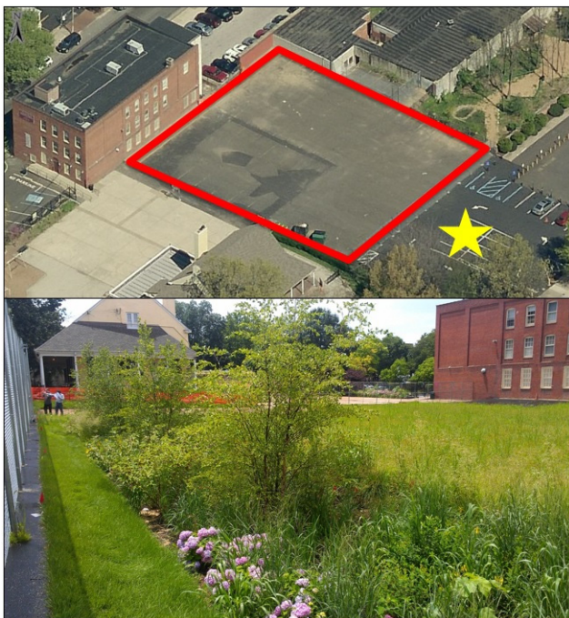
Figure 1. Philadelphia's Greene Street Friends School received one of the first SMIP grants awarded ($91,080 in 2012). The private school replaced a 16,330-square-foot parking area (top photo; depaved area denoted with red square) with a grassed play area. A rain garden (bottom photo) was added to manage runoff from an adjacent 9,280-square-foot parking area (top photo, denoted with yellow star). The completed project manages 18,912 gallons of runoff from a 1.5" storm and creates a greened open space for students and the community.
