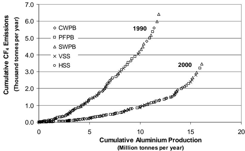
Figure 2. Comparison of Annual Emissions of CF<sub>4</sub> from Primary Aluminium Production Facilities for 1990 and 2000. (IAI, 2001)
