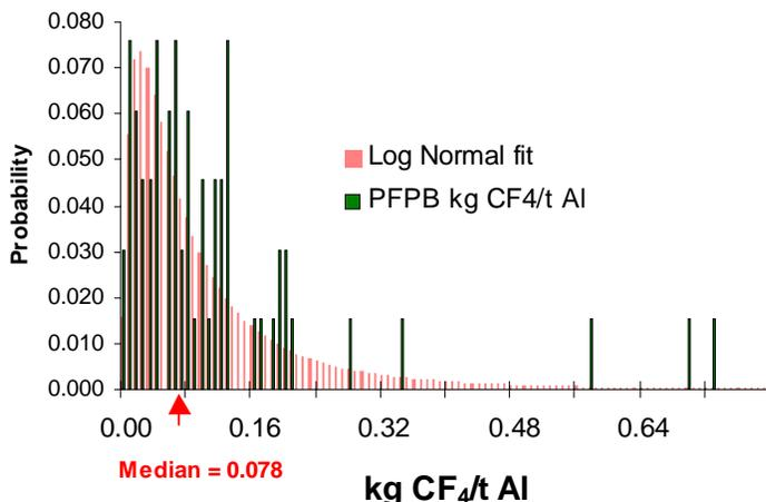
Figure 3. Specific CF<sub>4</sub> Emissions Performance of Point Fed Prebake Smelters
