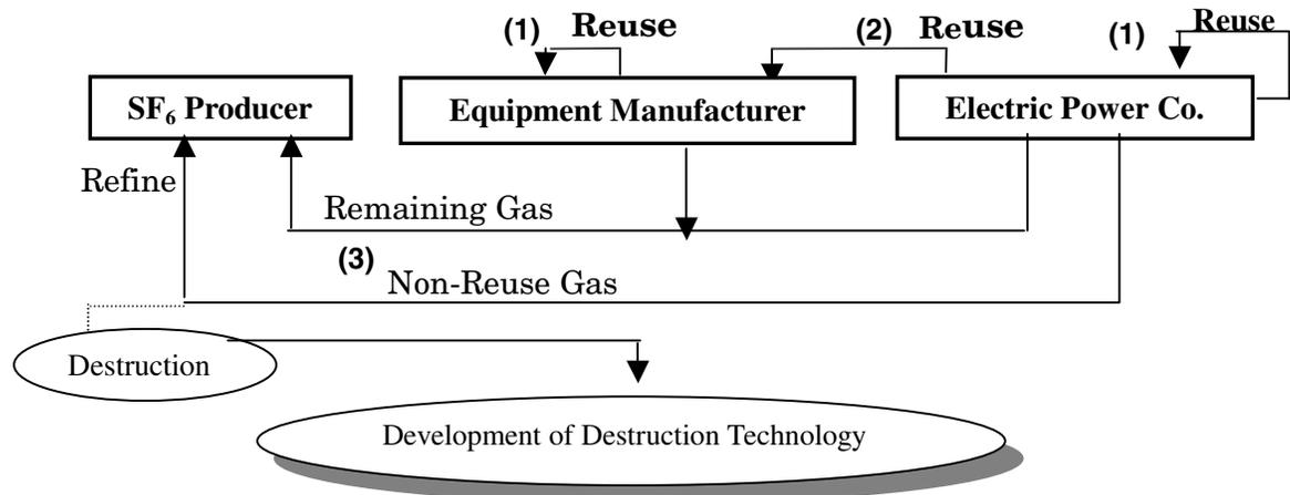
**Fig.6-1: SF<sub>6</sub> Gas Recycling Flow**
