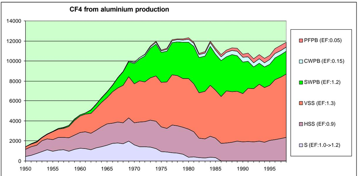
Figure 7. (a) Trend in global production of aluminium per type of process. (b) Trend in global emissions of CF<sub>4</sub> per type of process. (Source: EDGAR 3.0)
