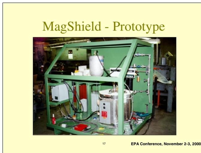
This shows the actual MagShield prototype system that was utilized at Lunt. The photo shows the furnace, feeder, and the dry air system.
