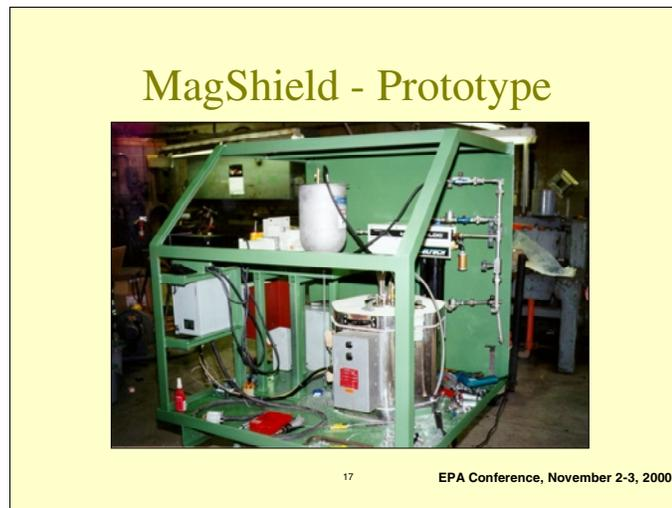
This shows the actual MagShield prototype system that was utilized at Lunt. The photo shows the furnace, feeder, and the dry air system.
