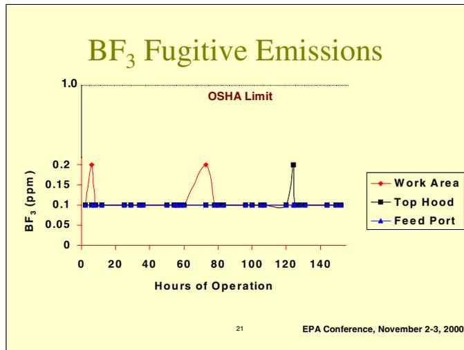
The BF<sub>3</sub> gas emissions were continuously monitored during our trials and the results are shown in this slide. The equipment used was the Enmet analyzer calibrated for 0-10 ppm level. A hood was provided over the work area and the hood exhaust gas concentration was measured. During all testing, gas concentrations were observed to be generally 10 times lower than the OSHA limit. The maximum concentration observed at any given time was approximately 0.2 ppm.
